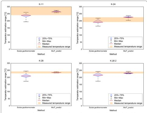
**Fig. 11** Comparison of conventional qualitative solute geothermometers based on back-calculated element concentrations using WATCH 2.4 (Bjarnason 2010) (cf. Appendix 4) with the end results of MulT\_predict (Fig. 7) for the wells at Krafla
