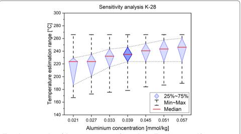
**Fig. 4** Sensitivity analysis of aluminium concentration for sample K-28. The value was varied from 0.009 to 0.117 mmol/kg in increments of 0.006 mmol/kg. The figure shows an extract of the data, where the aluminium concentration ranges from 0.021 to 0.057 mmol/kg in increments of 0.006 mmol/kg. The statistical minimum of the boxplot comparison is reached for a concentration of 0.039 mmol/kg highlighted in a darker blue colour
