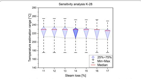
**Fig. 5** Sensitivity analysis of steam loss for sample K-28. The value was varied in increments of 1%. The figure shows an extract of the data, where the steam loss ranges from 11 to 17% in increments of 1%. For 14% steam loss, the statistical minimum of the boxplot comparison is reached; it is highlighted in a darker blue colour
