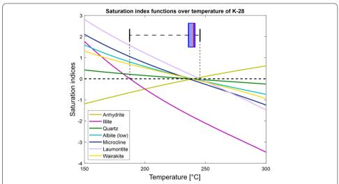
**Fig. 1** Example of the creation of an equilibrium temperature distribution box plot via the saturation indices over the temperature [ $^{\circ}$ C] of the basalt-specific mineral phases for sample K-28. The box plot includes the temperature values of each mineral where SI = 0 (intersection of the saturation index of a mineral phase and the equilibrium line)
