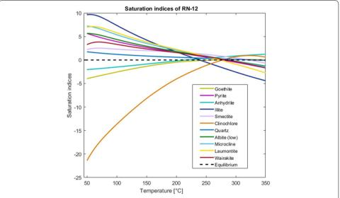
**Fig. 9** Initial saturation indices of the basalt-specific mineral set of RN-12 with a temperature range of up to  $350\,^{\circ}\mathrm{C}$  prior to the sensitivity analyses. Saturation curves approaching the critical point of water have to be used with care
