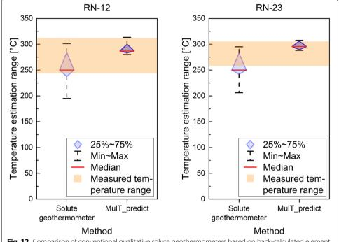
**Fig. 12** Comparison of conventional qualitative solute geothermometers based on back-calculated element concentrations using WATCH 2.4 (Bjarnason 2010) (cf. Appendix 4) with the end results of MuIT\_predict (Fig. 10) for the wells at Reykjanes
