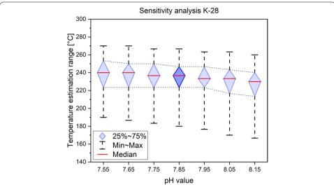
**Fig. 3** Sensitivity analysis of pH for sample K-28. The value was varied from 6.75 to 8.15 in increments of 0.1. The figure shows an extract of the data, where the pH value ranges from 7.55 to 8.15 in increments of 0.1. For pH 7.85, the statistical minimum of the boxplot comparison is reached; it is highlighted in a darker blue colour
