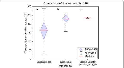
**Fig. 6** Comparison of an unspecific mineral set (a) with the developed basaltic set (b). The boxplot in the third column (c) is the result of the combination of the pH, aluminium concentration, and steam loss sensitivity analysis. All analyses are done separately under static conditions for the remaining parameters, and all best-fit parameters were combined afterwards
