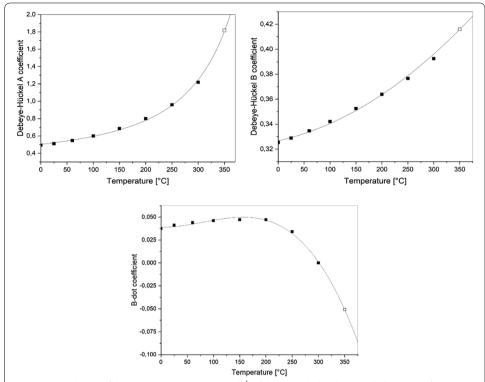
**Fig. 8** Extrapolation of the three parameters A, B, and  $\dot{\bf B}$  of the extended Debye–Hückel equation for temperatures beyond 300 °C. The values of the solid squares are acquired from the LLNL database in IPhreeqc. The hollowed squares are the results of a polynomial fit
