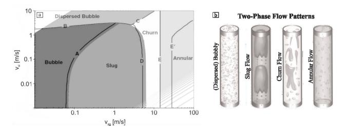
Figure 2: a) Validation of two-phase flow patterns. Simulated flow patterns (grey-shaded areas) as functions of superficial gas velocity  $v_{sg}$  and superficial liquid velocity  $v_{sl}$  match experimental data (field boundaries (black lines) according to Ishii and Hibiki, (2006)) in very good agreement. b) Scheme of different flow patterns ((disperse) bubbly, slug flow, churn flow and annular flow), which are evolving as a function of  $v_{sg}$  and  $v_{sl}$ .
