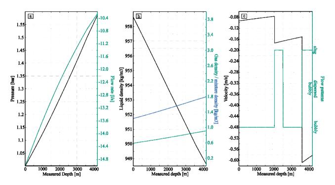
Figure 4: The pressure traverse and the flow rate are non-linear functions (Figure 4a), resulting from varying phase densities (Figure 4b) and changing volume ratios of the phases in the mixture. The decreasing pipe diameter causes increasing flow velocities which results in changing flow patterns alternating from bubbly to slug flow (Figure 4c).
