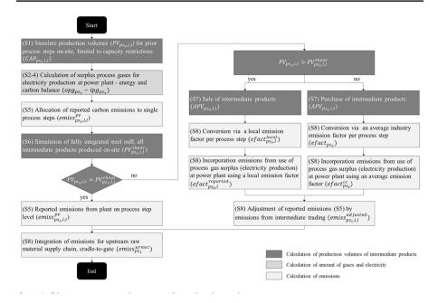
**Fig. 6** Flow chart of the site-specific CO<sub>2</sub>e approach for predefined calculation steps. *Note* The single steps (S1–8) correspond to Sect. 4.3.2.5 and will be further explained in the text
