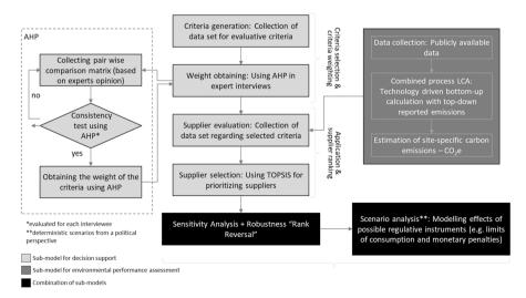
Fig. 1 Structure of the outlined model to integrate CO<sub>2</sub>e in the supplier selection process
