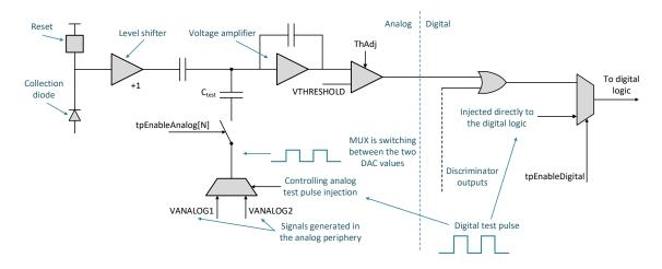
Figure 7.7 Test pulse injection in the CLICTD cell.
