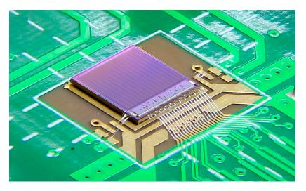
Figure 8.1 Photo of the CLICTD chip, wire bonded on the PCB.
