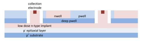
Figure 7.1 Process cross-section - continuous N-implant (not to scale).
