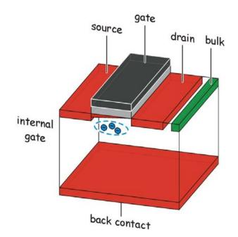
Figure 3.17 Schematic cross-section of a DEPFET pixel (from [83]).
