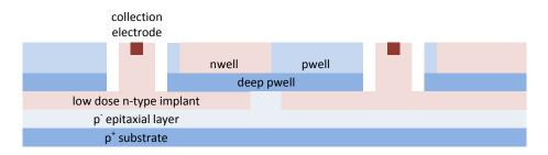
Figure 7.2 Process cross-section - gap in N-implant (not to scale).
