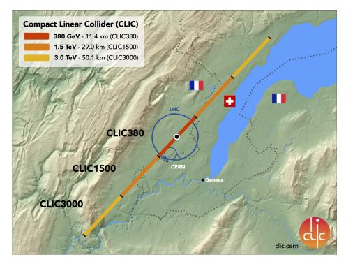
Figure 2.1 The CLIC accelerator footprint near CERN. The three foreseen energy stages are presented. From [5].
