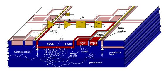
Figure 3.10 Schematic cross-section of a triple-well monolithic pixel. From [64].
