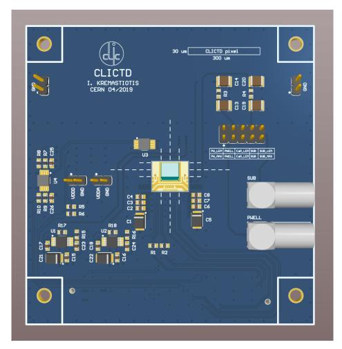
Figure A.5 Visualisation of the PCB designed for testing the CLICTD chip.
