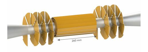
Figure 2.4 3-D model of the CLIC vertex detector. From [9].
