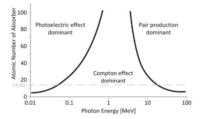
Figure 3.1 Interaction of photons with matter. From [12].
