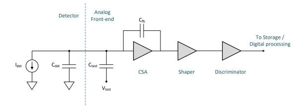
Figure 3.2 Block diagram of a typical processing chain in a particle detector.
