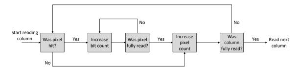
Figure 7.10 Algorithm diagram of the CLICTD End-of-Column block.
