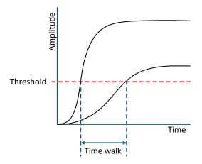
Figure 3.5 Time walk in a detector.
