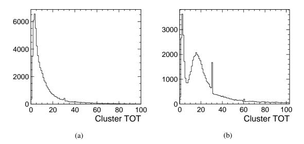
Figure 6.22 Resulting amplitude spectrum from a  $^{90}$ Sr source, for a capacitively coupled assembly with (a) a 20  $\Omega$ cm and (b) a 1000  $\Omega$ cm C3PD sensor. The peaks observed for the ToT value of 30 are resulting from single cluster hits where the ToT counter has saturated.
