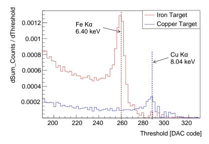
Figure 8.10 Fluorescence spectra using iron (red) and copper (blue) targets, measured with the CLICTD chip.
