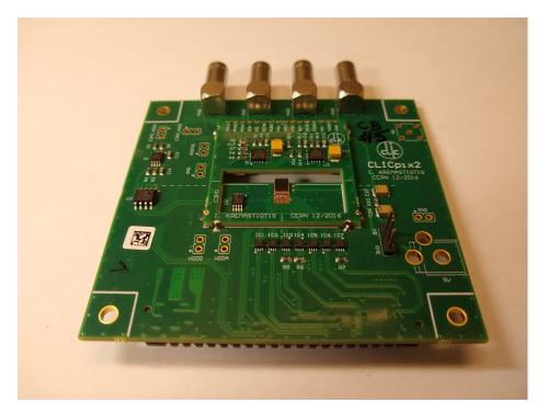
Figure A.4 Photo of the CLICpix2/C3PD PCB.
