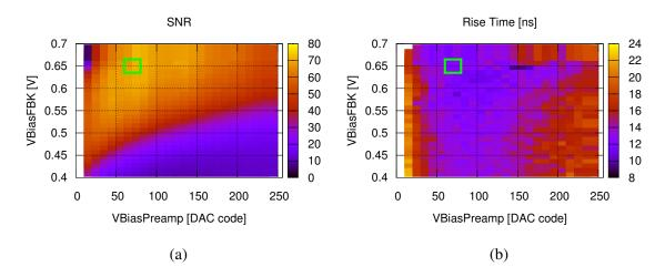
Figure 6.5 (a) Signal-to-noise ratio and (b) rise time as measured for different biasing points of the preamplifier and the feedback. The chosen operating point is marked in green.
