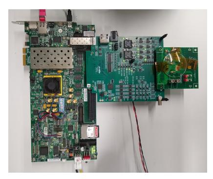
Figure 8.2 Photo of the CaRIBOu readout system for testing the CLICTD chip. From left to right: evaluation kit, CaR board, chip board with a CLICTD sample mounted on it.
