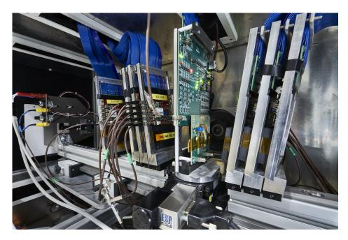
Figure 6.23 Measurement setup using the CLICdp Timepix3 telescope in the CERN SPS beamline. The DUT is shown in the middle, with four Timepix3 planes on the left and three on the right (© CERN).
