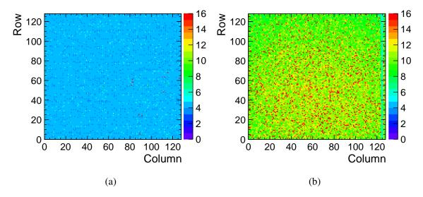
Figure 6.19 Noise width measured (in threshold DAC LSBs) in the CLICpix2 chip, with the C3PD sensor chip powered off (a) and on (b). From [106].
