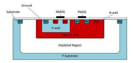
Figure 3.12 Schematic cross-section of a HV-CMOS process.
