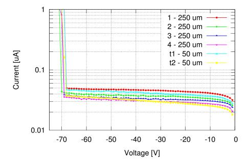
Figure 6.3 I-V curves of the measured C3PD chips. Samples with standard substrate resistivity ( $\sim 20~\Omega cm).$
