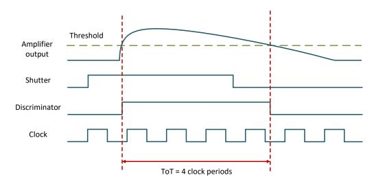
Figure 3.4 Timing diagram of a ToT measurement.
