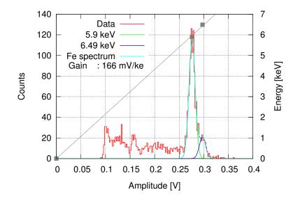
Figure 6.11 Resulting amplitude spectrum and double Gaussian fit from a <sup>55</sup>Fe source, for one of the monitored pixels of a high resistivity C3PD chip.
