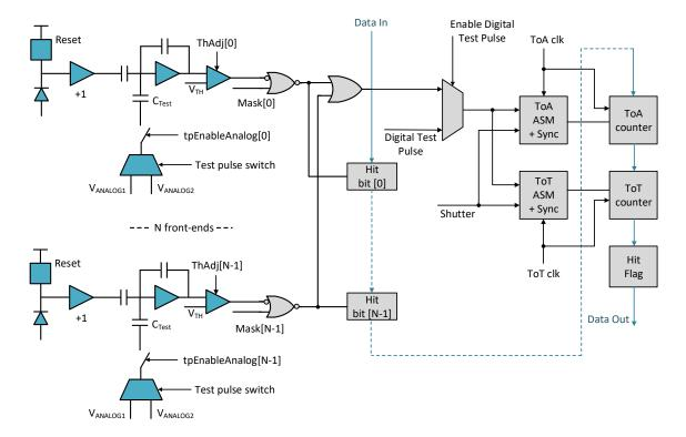
Figure 7.5 Block diagram of the CLICTD channel.
