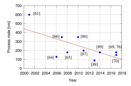
Figure 3.18 Different process nodes used for designing monolithic detectors over the years.
