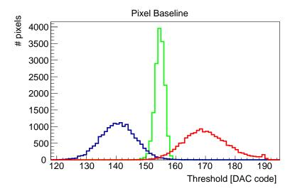
Figure 8.8 CLICTD threshold scan for minimum (blue), maximum (red) and equalised (green) local threshold tuning DAC code.
