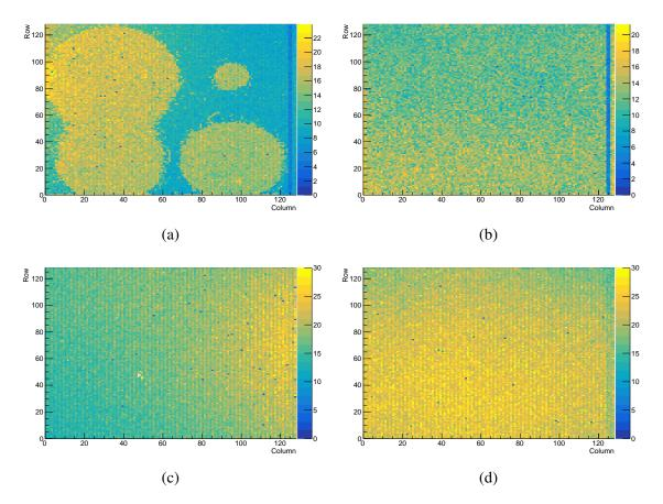
Figure 6.20 Hit maps acquired with the CLICpix2 readout chip, after injecting test pulses in the C3PD front-end. Figures (a) and (b) present two capacitively coupled assemblies with 20  $\Omega$ cm C3PD sensor chips and Figures (c) and (d) present two assemblies with 1 k $\Omega$ cm C3PD chips.
