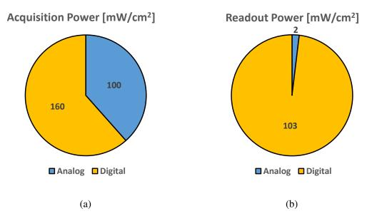
Figure 7.15 Contributions of the analog and digital power consumption of the CLICTD matrix (a) during acquisition and (b) during readout (simulated values).
