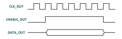
Figure 7.14 Timing diagram of the CLICTD readout.
