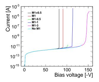
Figure 5.9 Leakage current as a function of the reverse bias voltage for different width of the metal contact. M1 is the original width of  $4.8 \,\mu m$ . From [99].
