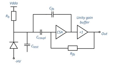
Figure 5.2 C3PD pixel block diagram.
