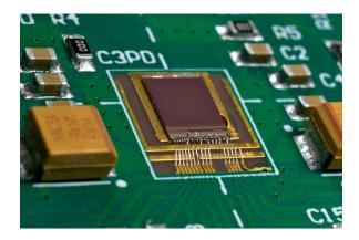
Figure 6.2 C3PD chip thinned down to 50 µm, mounted and wire-bonded on the PCB.
