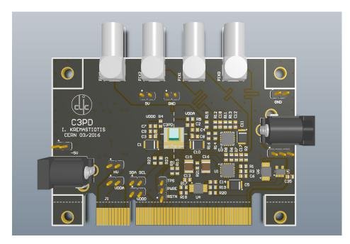
Figure A.1 Visualisation of the PCB designed for testing the C3PD chip in standalone mode.
