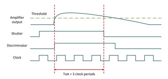
Figure 3.3 Timing diagram of a ToA measurement.
