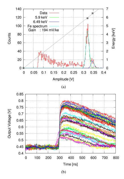
Figure 6.8 (a) Resulting amplitude spectrum and double Gaussian fit for one of the monitored pixels and (b) sample pulses from a  $^{55}$ Fe source.
