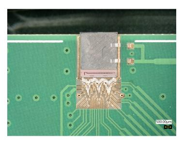
Figure 3.7 Photo of a hybrid pixel detector mounted on a PCB, with a silicon sensor bump-bonded on the CLICpix2 readout chip.
