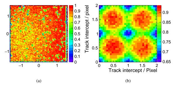
Figure 6.27 Efficiency measurement (a) across the matrix and (b) folded into a  $2 \times 2$  pixel array. From [106].
