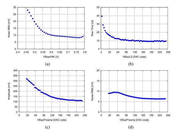
Figure 6.18 (a) Noise as a function of the feedback bias, (b) rise time as a function of the unity gain buffer bias, (c) output amplitude and (d) noise as a function of the charge sensitive amplifier bias for the measured C3PD chip. From [74].
