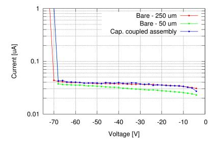
Figure 6.14 I-V curve for a C3PD chip in a capacitively coupled assembly, compared to the I-V curves for two bare chips: one 250 µm thick and one thinned down to 50 µm.
