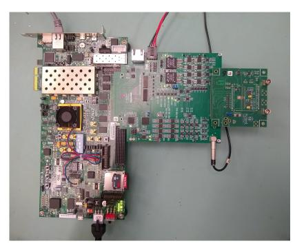
Figure 6.13 Photo of the CaRIBOu readout system for testing capacitively coupled assemblies with the CLICpix2 and C3PD chips. From left to right: evaluation kit, CaR board, chip-board with CLICpix2/C3PD assembly mounted on it.
