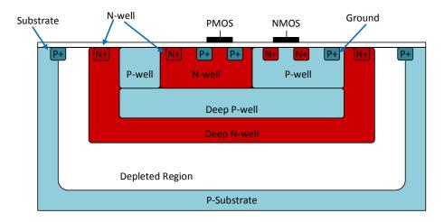
Figure 3.13 Schematic cross-section of a quadruple-well HV-CMOS process.
