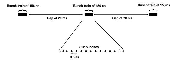
Figure 2.2 The CLIC beam structure (not to scale). From [7].
