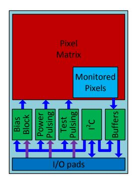
Figure 5.5 C3PD chip block diagram.
