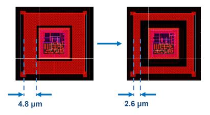
Figure 5.8 Modification in the metal contact of the HV-guardring in the C3PD pixel.
