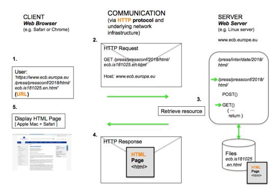
Figure 3.13: Example for a HTTP Communication
