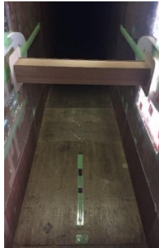
Figure 1. Section model for spring-supported tests mounted in Kyushu Institute Technology wind tunnel
