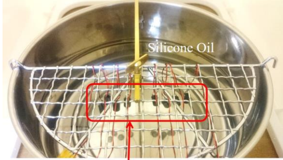
Capacitors under Test
