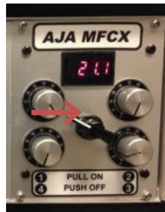
Fig. F.9 Gas shutter on
