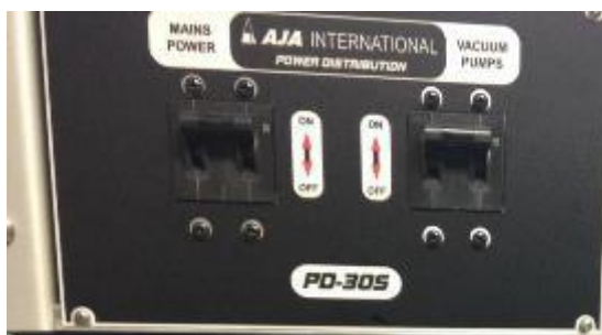
Fig. F.7 turn on the turbo pump
