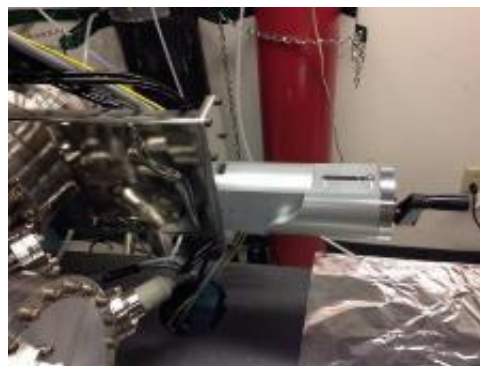
Fig. F.5 Turbo gate valve open (fully)
