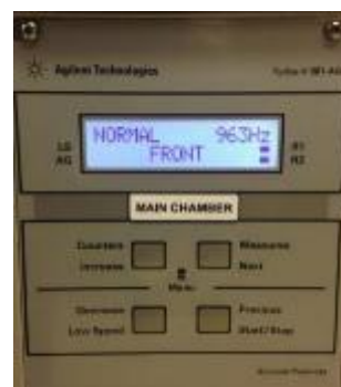
Fig. F.8 Frequency of the turbo pump should reach 963 Hz
