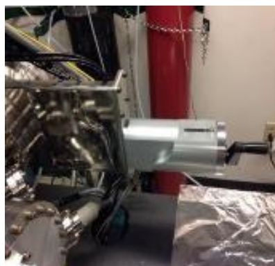
Fig. F.13 Change pressure to 3 \times 10^{-2} torr by changing gate valve position
