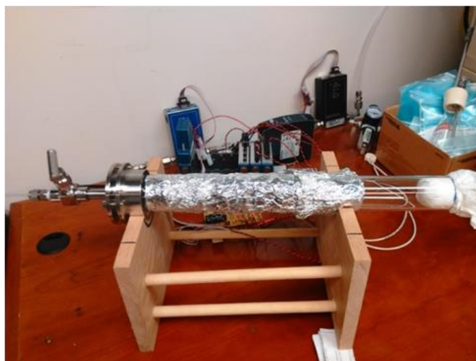
Figure 30. Schematic diagram of the second-generation gas sensor testing system (top) and photograph of the hardware setup (bottom).
