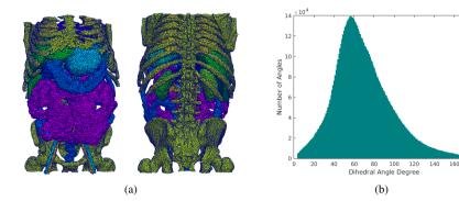
Fig. 1: (a) The final output mesh created by the algorithm. (b) Dihedral angle distribution of the final mesh.
