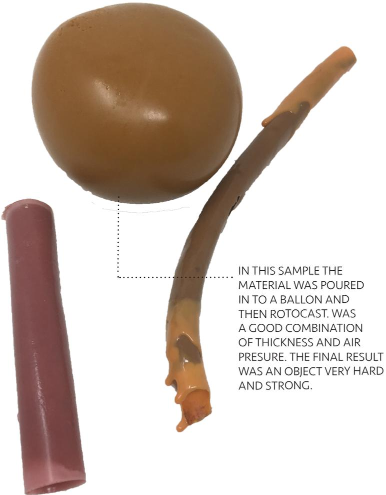
IN THIS SAMPLE THE MATERIAL WAS POURED IN TO A BALLON AND THEN ROTOCAST. WAS A GOOD COMBINATION OF THICKNESS AND AIR PRESURE. THE FINAL RESULT WAS AN OBJECT VERY HARD AND STRONG.
