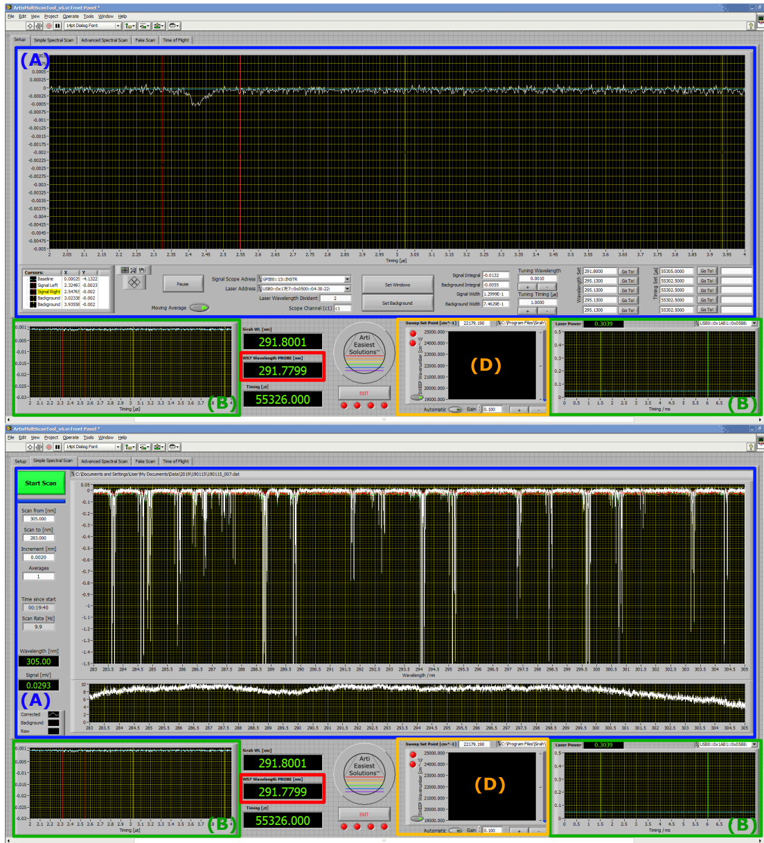
Figure A.1: Front panel of the Custom-made LABVIEW Environment showing the "Setup" and "Simple Spectral Scan" tab. The colored rectangles correspond to the marked features in Figure A.2. The blue (A) rectangle shows the main screen which can be switched using the tab control. Here the measured data is shown and measurement parameters are set. The green (B) rectangle depicts oscilloscope readings. On the left side the MCP oscilloscope is shown with integration borders for signal and background. The red rectangle shows the wavemeter reading. The yellow (D) rectangle shows the reading and control of the SWEEP laser stabilization.
