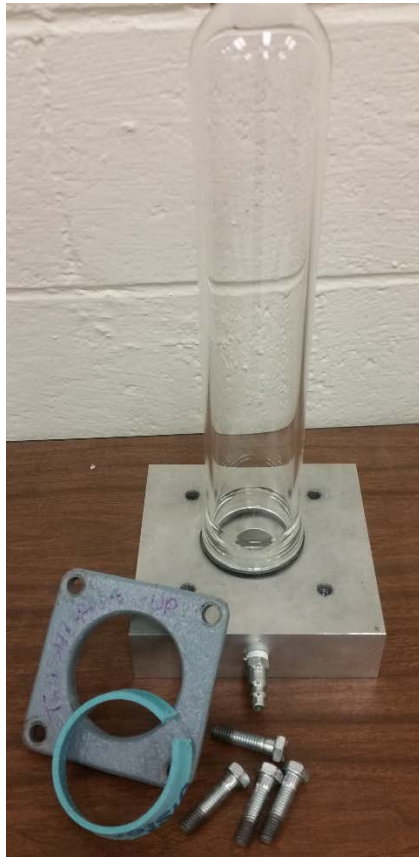
Figure 3-3: Pressure containment box prior to assembly.
