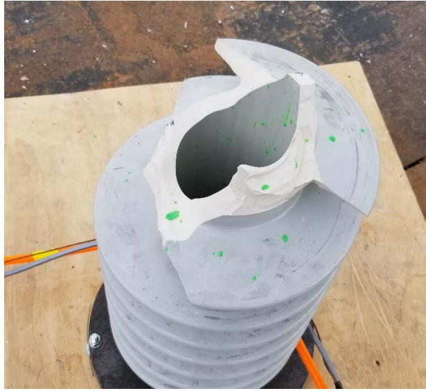
Figure 8-8 Pictures of (a) top and (b) bottom intact portions from bolt-mounted bushing.
