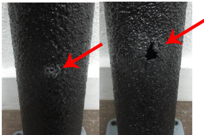
Figure 5-6: Images of post impact response from the 9x19 mm IMI FMJ test demonstrating fragmentation containment for coated cylinders: (left) bullet exit (right) bullet entrance.
