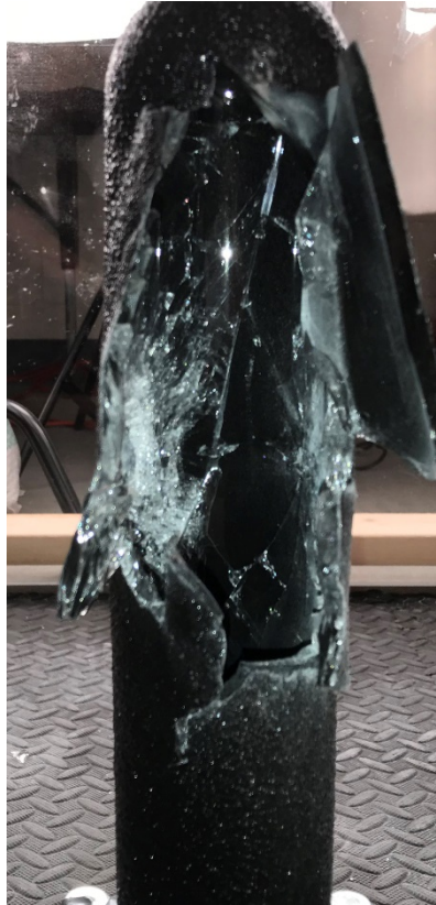
Figure 5-2: Side rupture of 1.43 mm thick coated cylinder.
