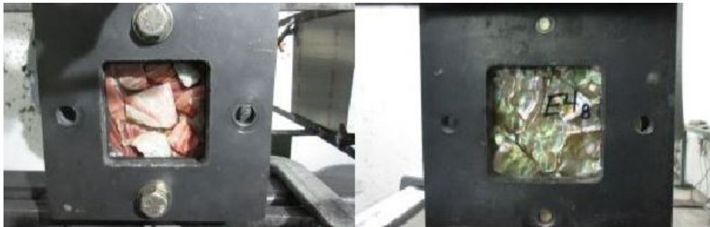
Figure 4-16: Oregon Ballistics test set-up for vacuum bagged abalone composite. Front view (left) and back view (right).
