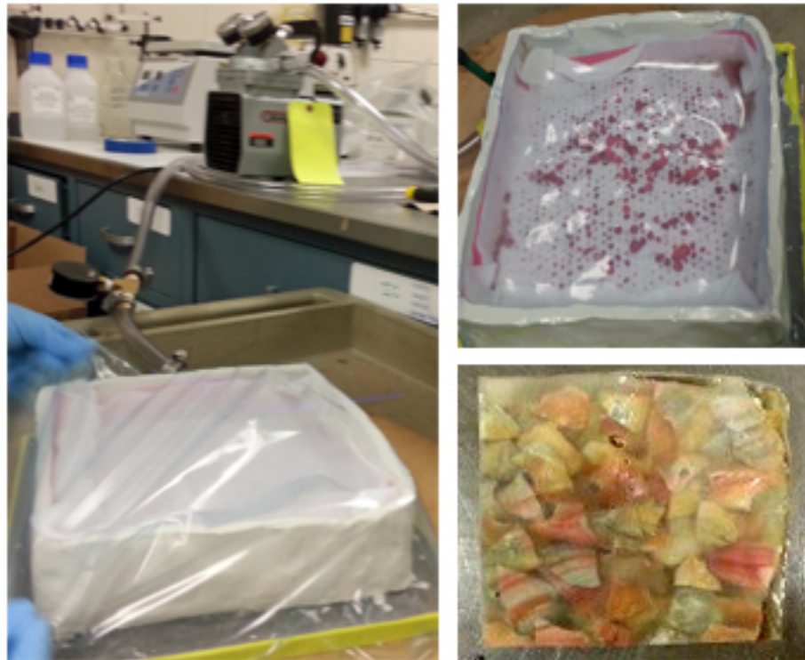
Figure 4-15: Vacuum bagging of abalone composites.
