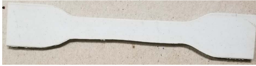
Figure 7-8: Elastomeric coating dogbone sample.
