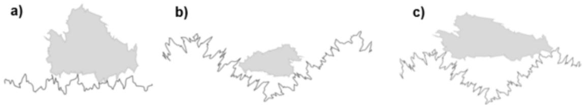
Figure 7.16. Schematics of a particle-surface interfacial contact, (a) particle size greater than the distance between two peaks, (b) particle size smaller than the distance between two peaks, (c) particle size similar to the distance between two peaks.
