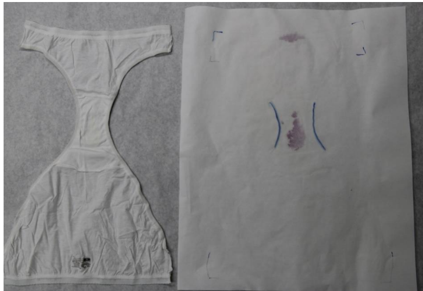
Figure 6: Acid phosphatase overlay used to detect seminal fluid stains on undergarments such as those submitted in cases of alleged sexual assault. The purple/pink color indicates the presumptive presence of acid phosphatase.
