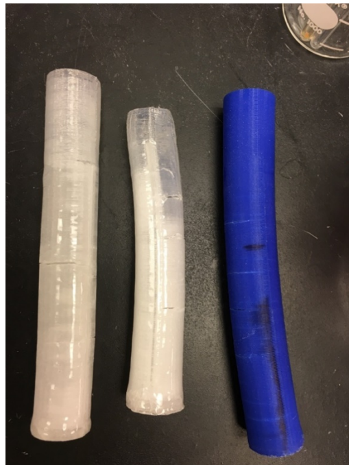
Figure 7.12 Acetone over-treated ABS tubes have shiny finish but may develop cracks after one year.
