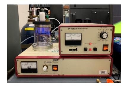
Figure 3. 14 Image of SPI-module sputter coater
