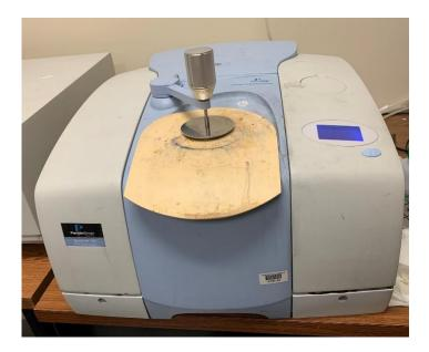
Figure 3. 11 Image of PerkinElmer Spectrum 100 FT-IR spectrometer
