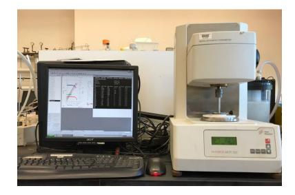
Figure 3. 5 Image of Physica MCR 300 rheometer under testing
