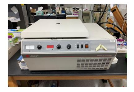
Figure 3. 21 Image of Beckman Coulter Allegra 6R Centrifuge
