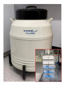
Figure 3. 18 Image of VWR CryoPro liquid nitrogen tank and the insert image shows the drawers in a rack system inside of the tank
