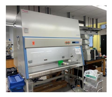
Figure 3. 17 Image of Thermo Scientific 1300 Series A2 Laminar-Flow Hood
