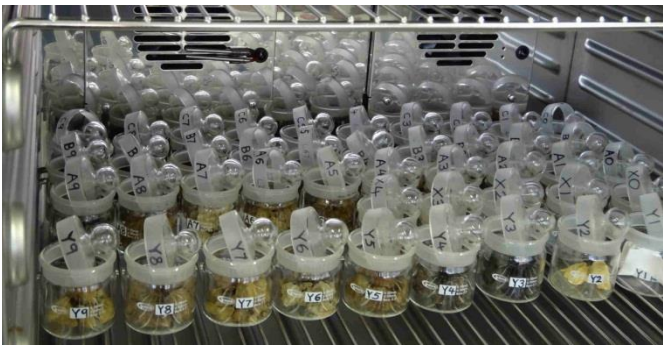
Figure 2 Thirty samples at 22MPa suction. Progress to equilibrium from natural moisture content
