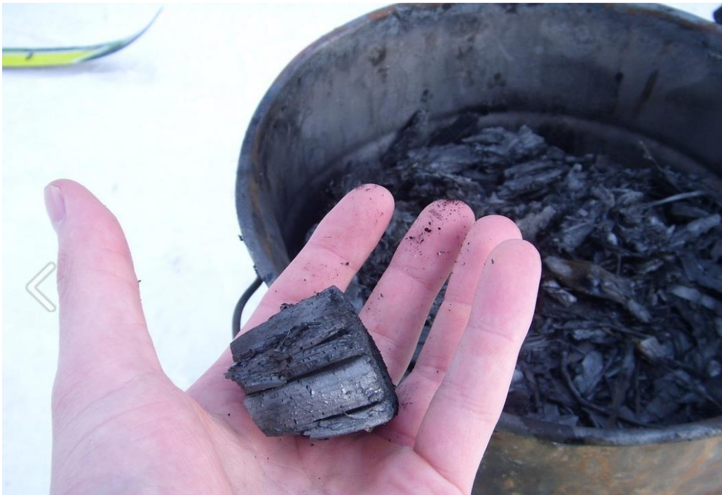
Figure 2 Biochar from the pyrolysis process. Image Credit: This file is licensed under the Creative Commons Attribution-Share Alike license and is attributed to Wikimedia username K.salo.85.
