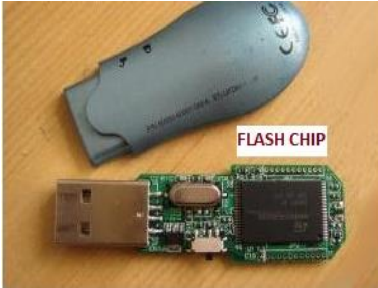
Figure 1: Flash chip on a USB Drive (Woodford, 2017)
