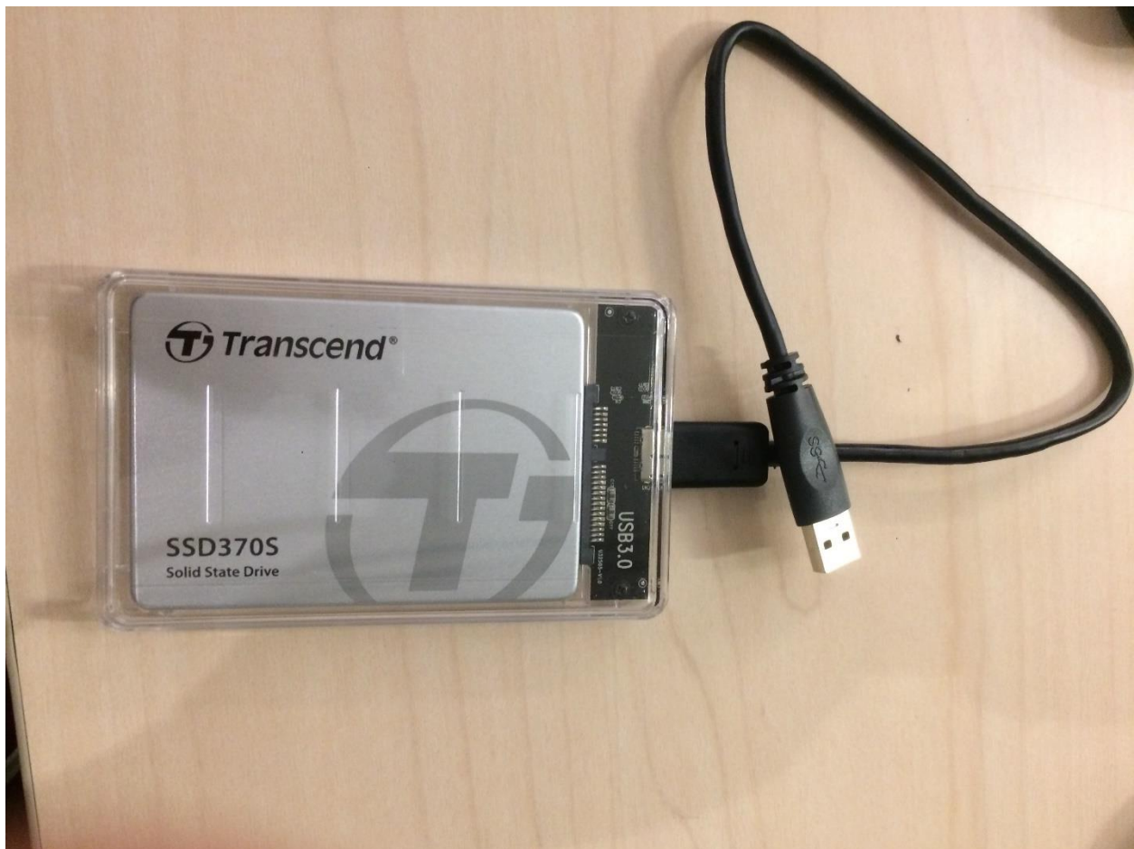
Figure 71: Externally connected SSD using SATA-USB device
