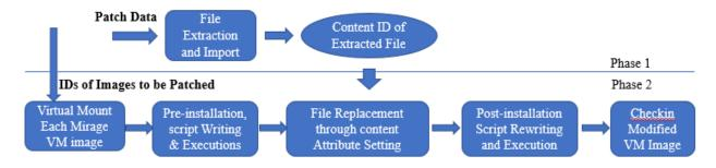
*Figure 9*: Batch Patching of Image via Mirage (Wu, Zhang, Wang, & Bala, 2010)
