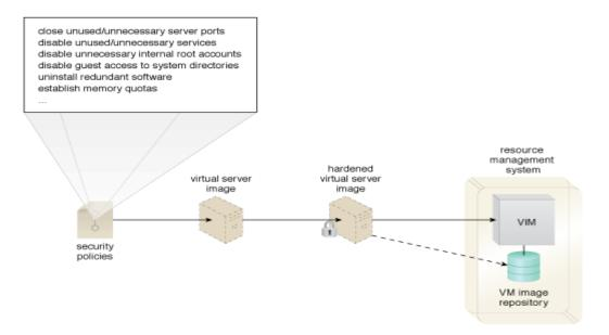
*Figure 14*: Hardening of the virtual image. ("Cloud Computing Design Patterns," n.d.)
