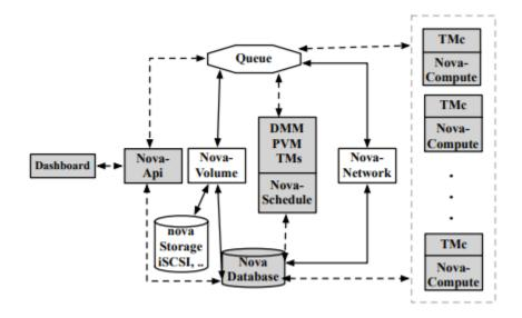
*Figure 12*: Implementation of Security on Demand on OpenStack Nova Components (Jamkhedkar et al., 2013)
