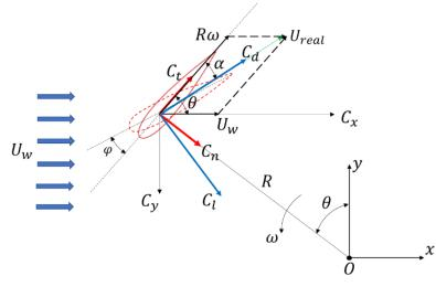
**Figure 39**. The velocity components and the hydrodynamic force acting on the blade (Zhang et al., 2019).
