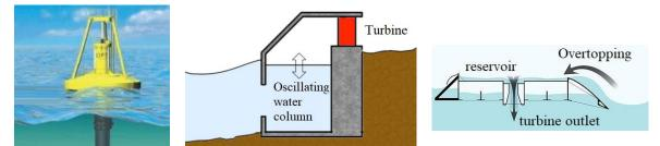
**Figure 2.** Wave Energy Converters: (left) Oscillating bodies (middle) Oscillating Water Columns, and (right) Overtopping device.
