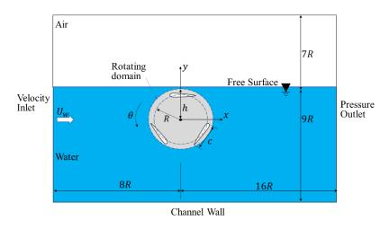
Figure 38. Schematic of flow around hydropower in shallow-tip immersion.
