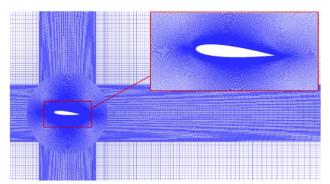
Figure 20. The grid system in entire domain and a close-up view of the grid near the hydrofoil for  $\alpha = +5^{\circ}$ .
