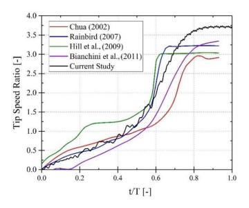
**Figure 16**. A comparison between the current study and the numerical data of Tip Speed Ratio versus non-dimensional time presented by Rainbird (2016), Hill et al. (2009), Bianchini et al. (2011), and Chua (2002).
