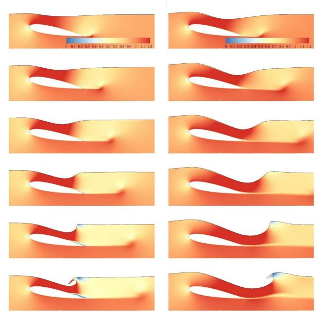
**Figure 25.** The evolution of free surface including wave formation for (left) h/c = 0.3, Fr = 0.3, and  $\alpha = +10^{\circ}$ ; (right) h/c = 0.3, Fr = 0.6, and  $\alpha = +10^{\circ}$ . Contours are colored by normalized velocity magnitude.
