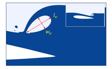
Figure 35. Wave breaking at the plunge point and cavity shape parameters.
