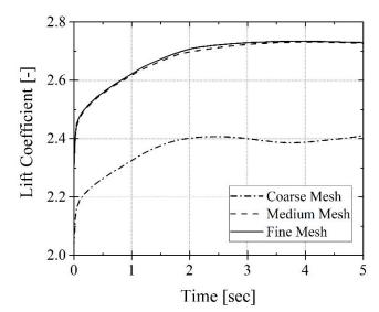
Figure 11. The time history of lift coefficient for three different grid systems.
