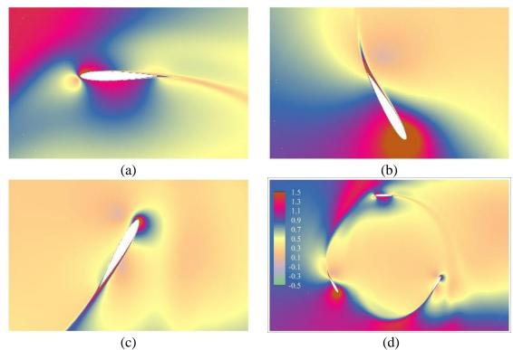
**Figure 15**. The velocity contour at different azimuthal angles (a)  $\theta = 0^{\circ}$  (b)  $\theta = 120^{\circ}$  (c)  $\theta = 240^{\circ}$ , and (d) overall view.
