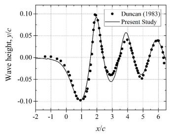
Figure 6. The wave elevations for NACA0012 hydrofoil at h/c = 0.91 and Fr = 0.57 compared against experiment results by Duncan (1983).
