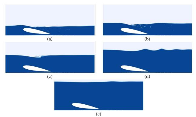
**Figure 23**. Instantaneous contours of the water volume fraction for the Fr = 0.3,  $\alpha = +10^{\circ}$ , and various submerged depths (a) h/c = 0.2, (b) h/c = 0.3, (c) h/c = 0.5, (d) h/c = 0.7, and (e) h/c = 0.9.
