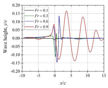
Figure 34. The wave profile before breaking for Froude numbers at  $\alpha = +5^{\circ}$  and h/c = 0.3.
