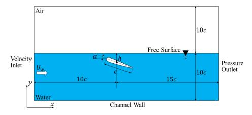
Figure 19. Schematic of the hydrofoil under free surface.4.1. Mathematical modeling of flow over hydrofoil
