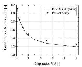
**Figure 9**. Comparison of local Froude number  $(Fr_L)$  as function of gap ratio (the Froude number based on maximum velocity in the region directly above the cylinder) against the results from Reichl et al. (2005).
