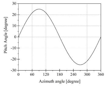
Figure 52. Pitch angle of blade versus azimuthal angles.
