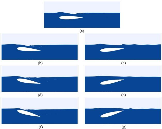
**Figure 22.** Instantaneous contour of the water volume fraction for the h/c = 0.2, Fr = 0.3 and various angles of attack (a)  $\alpha = 0^{\circ}$ , (b)  $\alpha = +5^{\circ}$ , (c)  $\alpha = -5^{\circ}$ , (d)  $\alpha = +10^{\circ}$ , (e)  $\alpha = -10^{\circ}$ , (f)  $\alpha = +15^{\circ}$ , (g)  $\alpha = -15^{\circ}$ .
