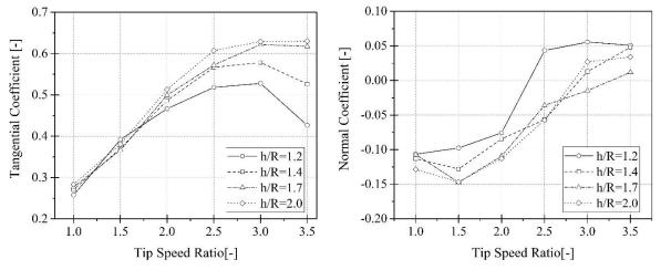
Figure 48. Mean tangential (top) and normal (bottom) coefficient for various tip speed ratio at four different submerged depths.
