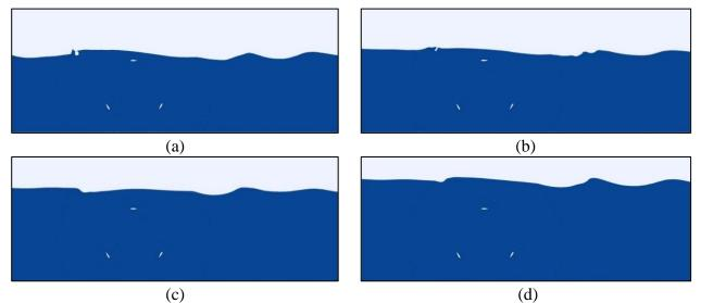
**Figure 41**. Instantaneous contours of the water volume fraction for tip speed ratio of  $\lambda = 2$  at different submerged depths of (a) h/R = 1.2; (b) h/R = 1.4; (c) h/R = 1.7; (d) and h/R = 2.
