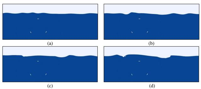
**Figure 43**. Instantaneous contours of the water volume fraction for submerged depth of h/R=1.7 at different tip speed ratios (a)  $\lambda = 1$ ; (b)  $\lambda = 1.5$ ; (c)  $\lambda = 2$ ; (d)  $\lambda = 2.5$ .
