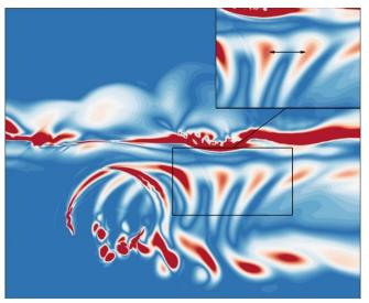
Figure 46. Vorticity magnitude in the near wake of the turbine for submerged depth of h/R = 1.7, and tip speed ratio of  $\lambda = 2$ .
