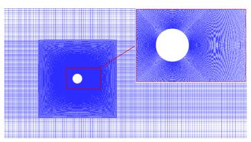
**Figure 7**. The grid system in entire domain and a close-up view of the grid near the cylinder for validation.
