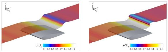
**Figure 21.** Instantaneous contour of the water volume fraction colored with velocity magnitude for the h/c = 0.3, Fr = 0.3 and 3 angle of attack  $\alpha = +5^{\circ}$ .
