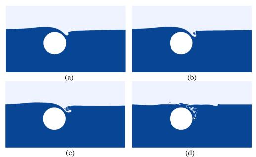
Figure 10. Jet formation over the cylinder for case of h/d = 0.1 and  $Fr_L = 0.3$  at time of (a) 0.5s, (b) 0.7s, (c) 1.1s, and (d) 2.1s.
