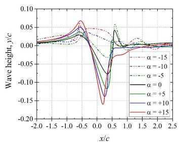
**Figure 30**. The wave profile before breaking for different angles of attack at h/c = 0.2 and Fr = 0.3.
