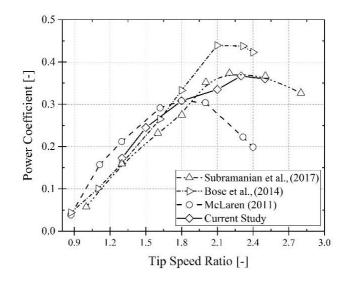
**Figure 14**. A comparison between the current study and the numerical data of the power coefficient with Tip Speed Ratio presented by Subramanian et al. (2017), McLaren (2011), and Bose et al. (2014).
