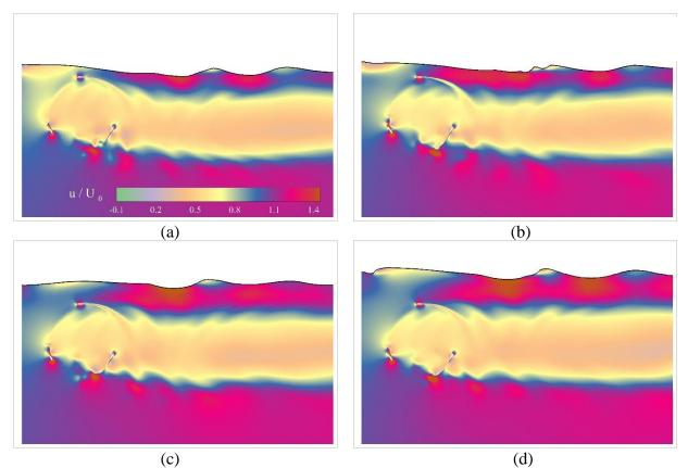
**Figure 44**. Normalized velocity contour for tip speed ratio  $\lambda = 2$  at different submerged depths of (a) h/R = 1.2; (b) h/R = 1.4; (c) h/R = 1.7; (d) and h/R = 2.
