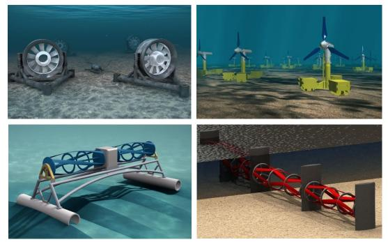
**Figure 3**. Example of horizontal axis (top) and vertical axis (bottom) hydropower turbines.
