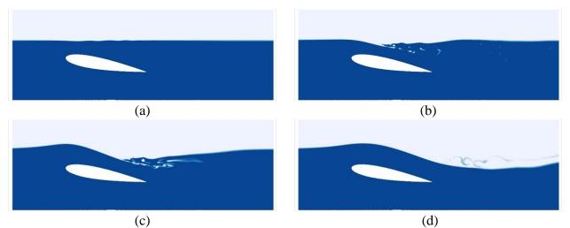
**Figure 24.** Instantaneous contours of the water volume fraction for the h/c = 0.3,  $\alpha = +10^{\circ}$ , and various Froude numbers (a) Fr = 0.1, (b) Fr = 0.3, (c) Fr = 0.6, and (d) Fr = 0.9.
