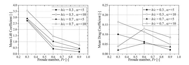
Figure 29. The average (top) lift and (bottom) drag coefficient versus Froude number for different submerged depths and angles of attack.4.4. Wave profile over free surface
