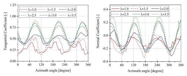
Figure 47. The instantaneous of tangential (left) and normal (right) coefficients for various tip speed ratio at submerged depth h/R = 1.7.
