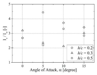
Figure 36. Measured cavity length to width ratio as a function of angle of attack for Fr = 0.3 and various submerged depths.
