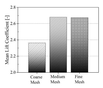
Figure 12. The average lift coefficient for three different grid systems.
