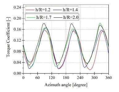
Figure 49. Torque coefficient versus azimuth angle at tip speed ratio of  $\lambda = 2$  for various submerged depths.
