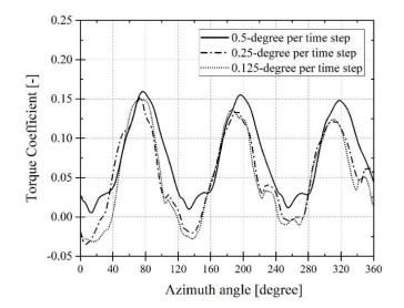
**Figure 18**. The variation of torque coefficient versus Azimuth angle at three different time steps of hydropower turbine.
