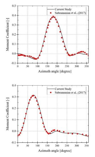
**Figure 13**. A comparison between the current study and the numerical data of the moment coefficient of blade1 in 2-blade (top) and 3-blade (bottom) turbine with tip speed ratio of 2.5 presented by Subramanian et al. (2017).
