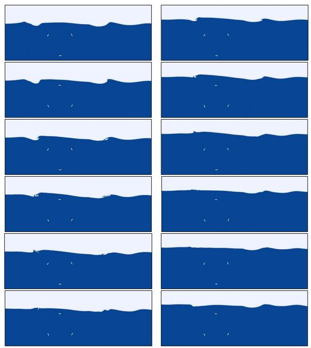
**Figure 42**. Instantaneous contours of the water volume fraction for tip speed ratio of  $\lambda = 2$  at submergence depth (left) h/R=1.4, and (right) h/R=1.7 at every 60-degree.
