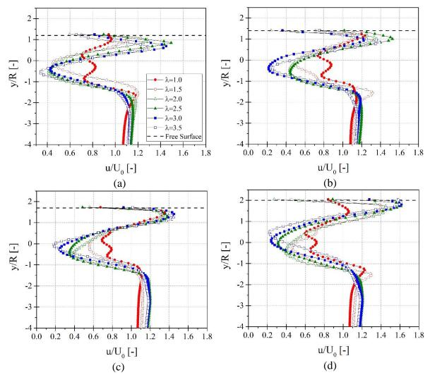
**Figure 45**. Comparison of the normalized velocity profile at x/R = 5 wake structure for various TSR at (a) h/R = 1.2; (b) h/R = 1.4; (c) h/R = 1.7; and (d) h/R = 2.
