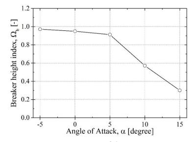
Figure 32. The variation of break height index for h/c = 0.2 with angle of attack.
