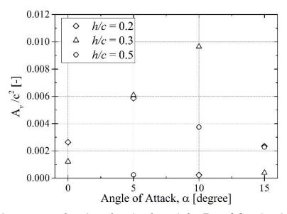
Figure 37. Cavity areas as a function of angle of attack for Fr = 0.3 and various submerged depths.
