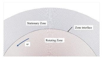
Figure 5. The concept of sliding mesh technique using in flow over rotating turbine. 2.5. Six DOFs
