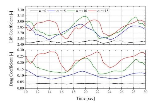
Figure 28. The instantaneous (top) lift and (bottom) drag coefficients for various angles of attack at h/c = 0.3 and Fr = 0.3.
