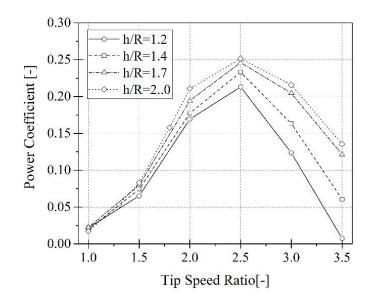
Figure 50. Power coefficient versus tip speed ratio for various submerged depths.
