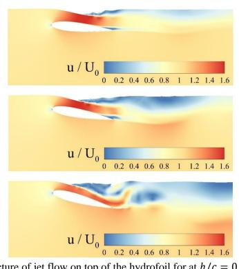
**Figure 26**. The structure of jet flow on top of the hydrofoil for at h/c = 0.3, Fr = 0.3 and different angles of attack (top)  $\alpha = +5^{\circ}$ , (middle)  $\alpha = +10^{\circ}$ , and (bottom)  $\alpha = +15^{\circ}$ .
