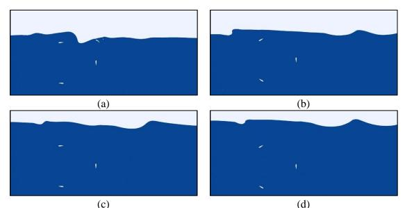
Figure 53. The comparison of free surface between variable pitch (left) and fixed pitch (right) at submerged depths of (a-b) h/R = 1.2; and (c-d) h/R = 2.
