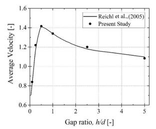
**Figure 8**. Comparison of average velocity direct above the cylinder as a function of gap ratio at the point of maximum lift against the results from Reichl et al. (2005).
