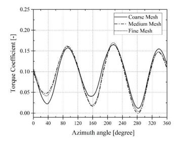
Figure 17. The variation of torque coefficient versus Azimuth angle at three different grid systems of hydropower turbine.
