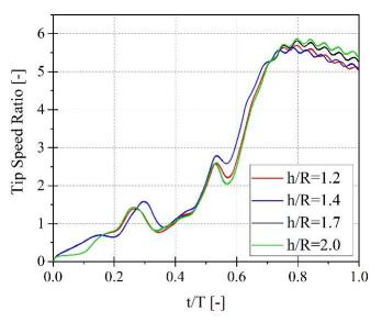
**Figure 51**. Tip speed ratio time series during turbine start-up for different submerged depths.
