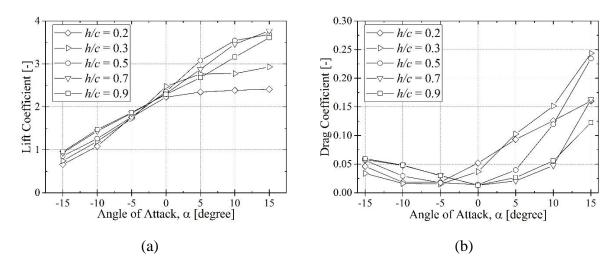
Figure 27. The average (left) Lift and (right) Drag coefficient versus angle of attack for various submerged depths and Fr = 0.3.
