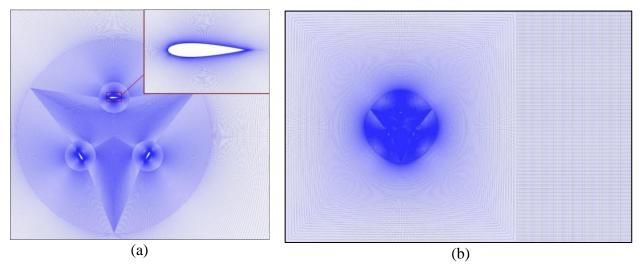
**Figure 40**. The structural grid system (a) around blade and rotation domain; (b) view of whole computational domain.
