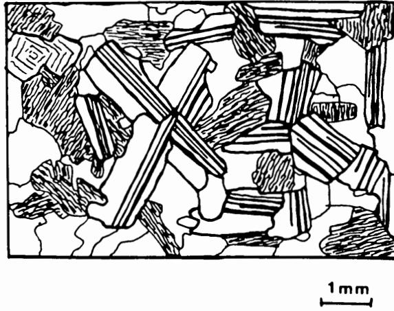
Figure 23. Euhedral plagioclase laths and hornblende grains randomly oriented in a primary igneous texture. Sample # 60, from Holden Lake pluton.
