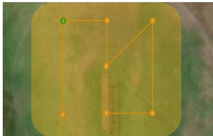
Figure 4.7: Effective survey area and survey waypoints expanded about the drop-zone's approximate location (waypoint 8)
