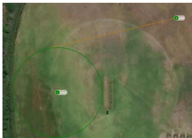
Figure 4.10: Fixed-wing landing waypoints
