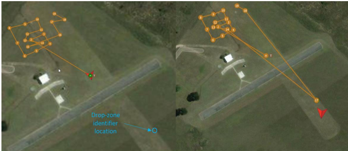
Figure 8.29: GCS mission map view of the second onboard integrated testing of the vision system and autonomous flight control system
