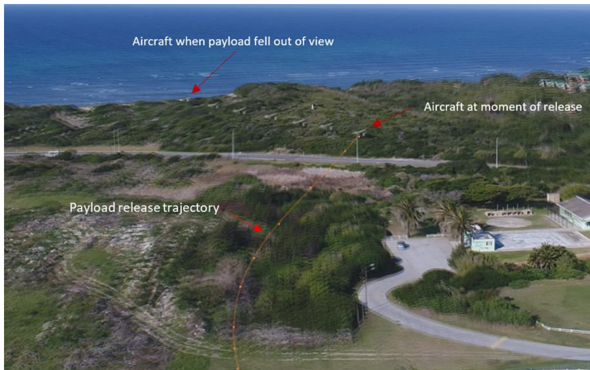
Figure 8.36: Stitched image illustrating the payload release trajectory and aircraft flight progression during payload release testing
