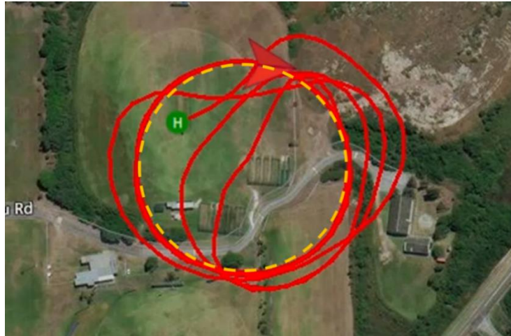
Figure 8.2: Autonomous flight control loiter with theoretical loiter circle overlaid
