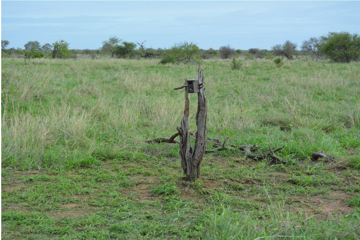
Figure 4: A typical example of camera traps fitting at the sites. Cameras were fitted to trees or tree stumps along the edge of the plot where possible, at 0.5 m to 1 m above ground to have the best view of the plot. The treatment edge is also visible along the back and sides of the camera, with uncut regrowth in the background.
