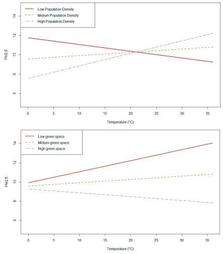
Figure 4. Effect of interaction (a) between temperature and population density (top); and (b) between temperature and green space (bottom) on  $PM_{2.5}$ .
