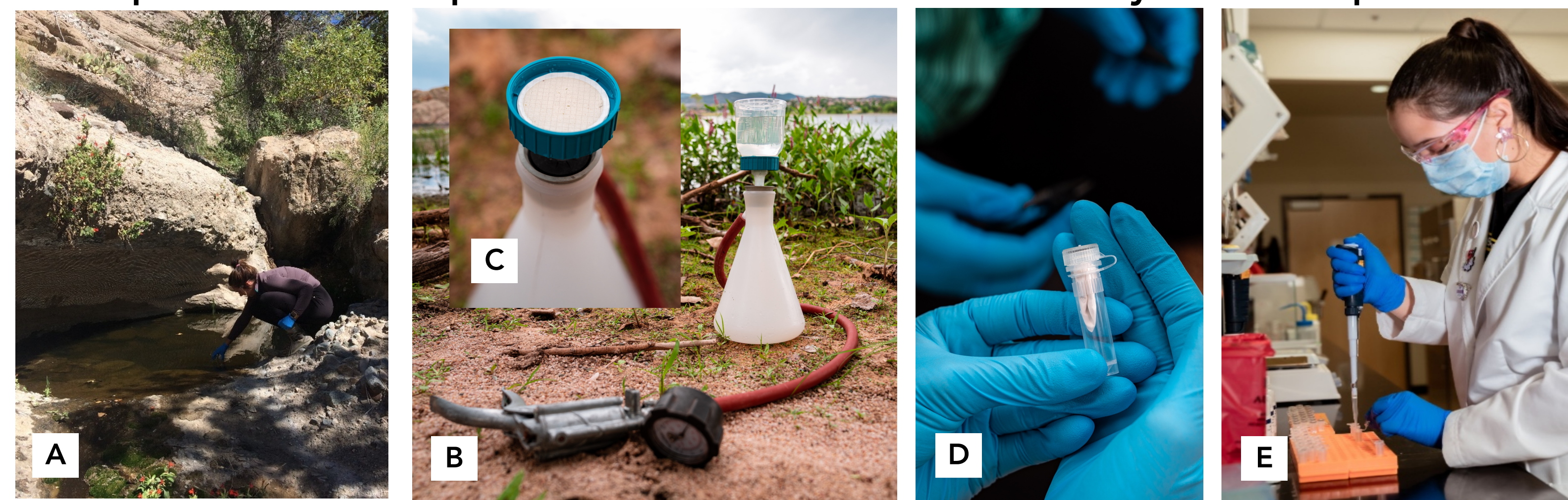
Fig. 2. (A) A sample being collected at Box Canyon Spring, (B) the sample filtration set-up in the field, (C) a sample filter, (D) filter in a sterile tube for transport to the lab, and (E) Completing eDNA extraction in the lab.
