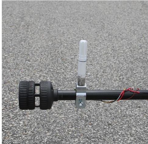
Figure 4. Boom mounted FT205 acoustic resonance wind sensor by FT Technologies that measures the vertical ( w ) wind component, along with the adjacent mounting of the HygroClip HC2A-S for vertical flux calculations.
