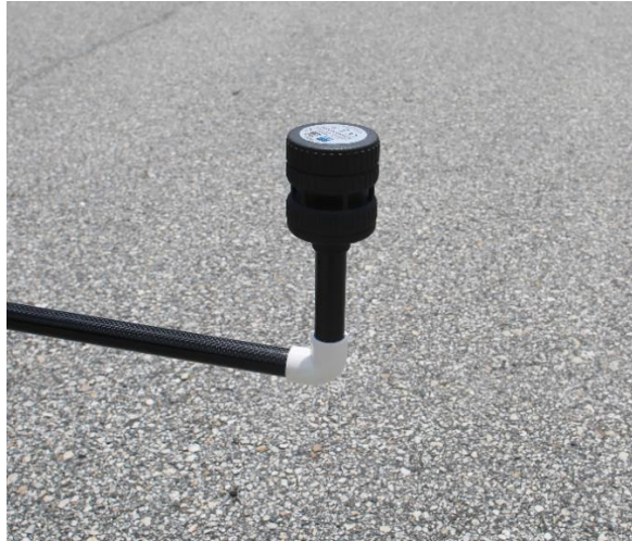
Figure 2. Pole mounted FT205 acoustic resonance wind sensor by FT Technologies that is used to measure horizontal (u,v) wind components.
