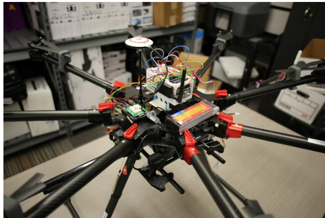
Figure 3. Pixhawk flight controller, sensor suite microcontroller, and telemetry.
