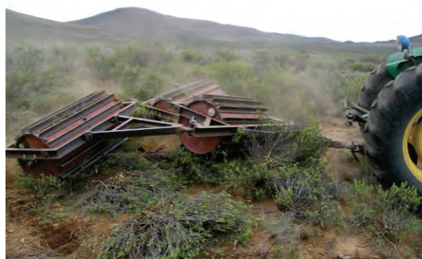
Figure 1. Knife roller in action. The initial concept of one long roller was modified to be able to work in gullies.
