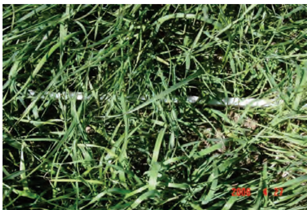
Figure 1. Determining photosynthetically active radiation (PAR) intercepted by a medium density Dactylis glomerata canopy with a sunfleck PAR ceptometer.
