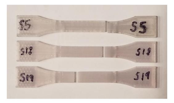
Figure 17: Three batch "S" specimens which exhibiting fracture patterns in the gauge length
