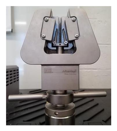
Figure 25: MTS Advantage wedge-action grips
