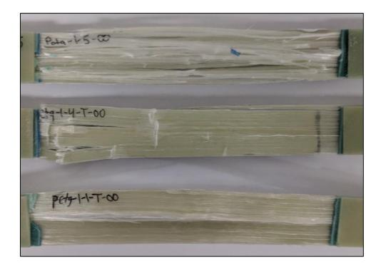
Figure 31: E-glass/PETg UD Multiple Failures Long. Tension Samples
