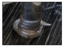
Figure 94: Failed Mobile Welded Single TP Stud Shear Specimen
