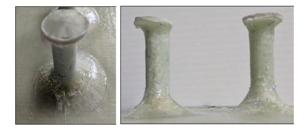
Figure 83: Untested Vacuum Infused Elium Shear Studs
