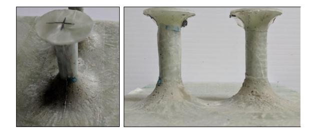
Figure 112: Tested E-glass/Elium Shear Studs (Broken out of Concrete)
