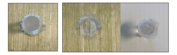
Figure 88: Failed Instron Welded Double TP Stud Shear Specimen (side 1)
