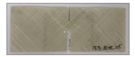
Figure 33: E-glass/PETg Bias Modified N2 Tension Sample
