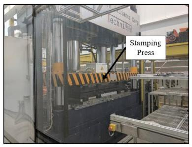
Figure 11: 650 Metric Ton Utah Hydraulic Press
