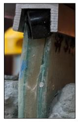
Figure 106: Elium Concrete-CFRTP Stud Specimen 5 Failure Mode
