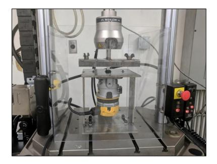
Figure 73: Instron Welding Setup
