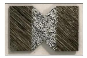
Figure 66: E-glass/PETg [+/- 45 90 0]s Failed In-Plane Shear Sample
