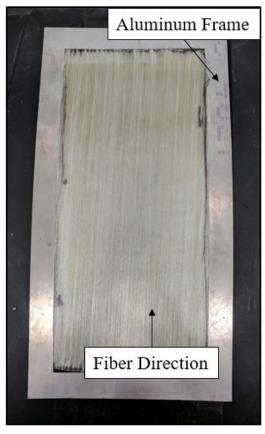
Figure 14: Pre-Consolidated PETg Prepreg in Aluminum Consolidation Frame
