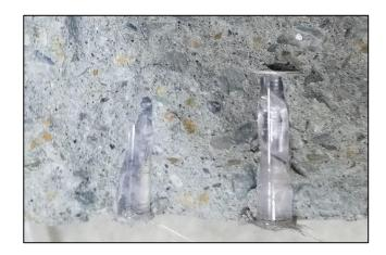
Figure 110: PETg Neat-resin PETg Shear Studs Embedded in Concrete
