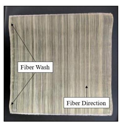
Figure 13: Improved UD PETg Thermoformed Panel
