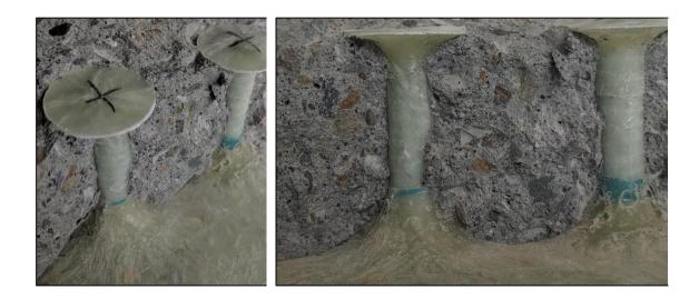
Figure 111: E-glass/Elium Shear Studs Embedded in Concrete
