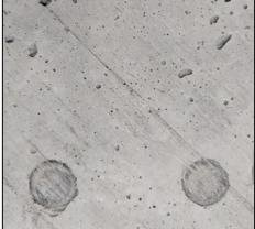
Figure 103: Failed PETg Concrete-TP Stud Specimen (Concrete side)
