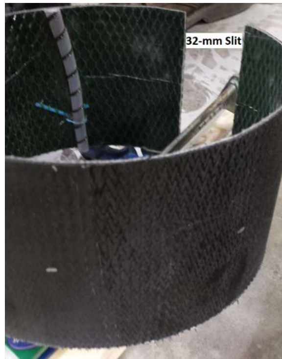
Figure 2-2 32-mm Longitudinal Slit in Collar
