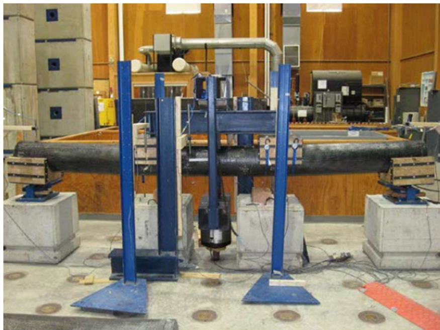
Figure 2-6. Four-Point Bend Test of Control Beam, (Dagher et al. 2012)
