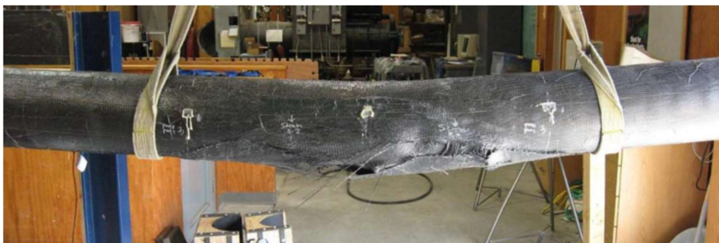
(c) Control Beam: Typical Specimen Failure Mode
