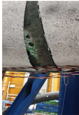
(b) Spliced Beam with Collar: FRP Shell Debonding
