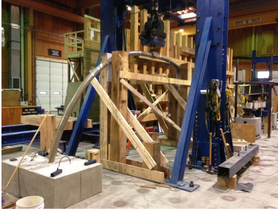
Figure 3-11. Photo of Arch in Test Device
