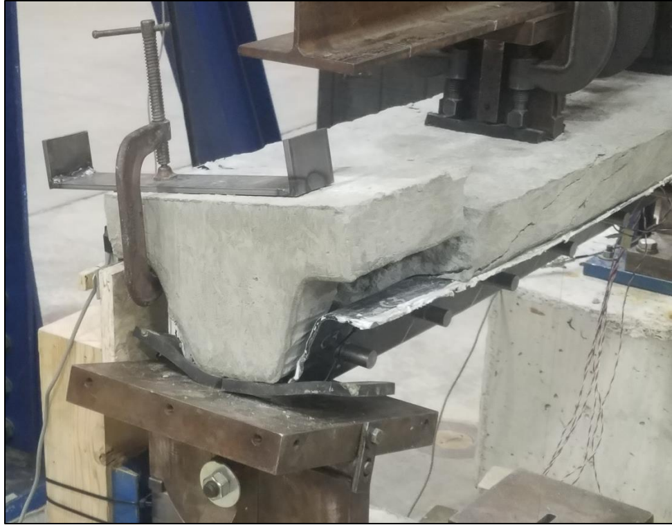
Figure 66: Failure of hybrid beam specimen
