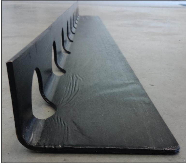
Figure 87: Misaligned angle with holes cut before forming
