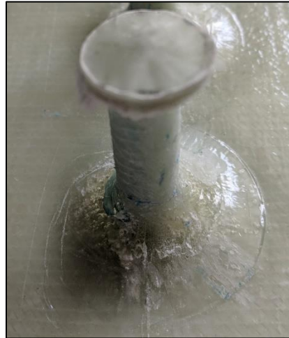
Figure 5: E-glass/Elium infused shear stud [7]
