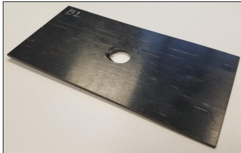
Figure 15: Failed bearing specimen
