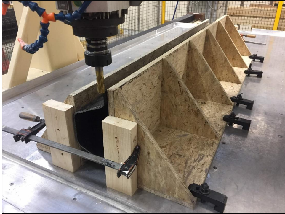
Figure 49: Bearing holes being cut into a corrugated panel
