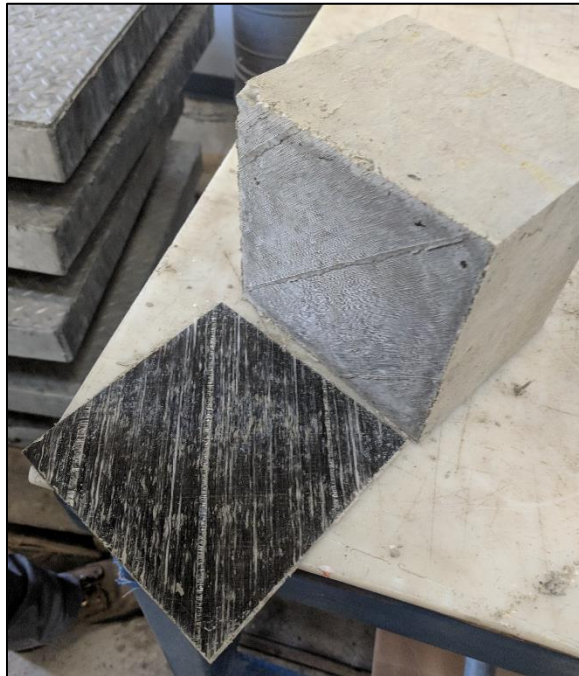
Figure 17: Test of mold release before (left) and after (right) breaking the bond
