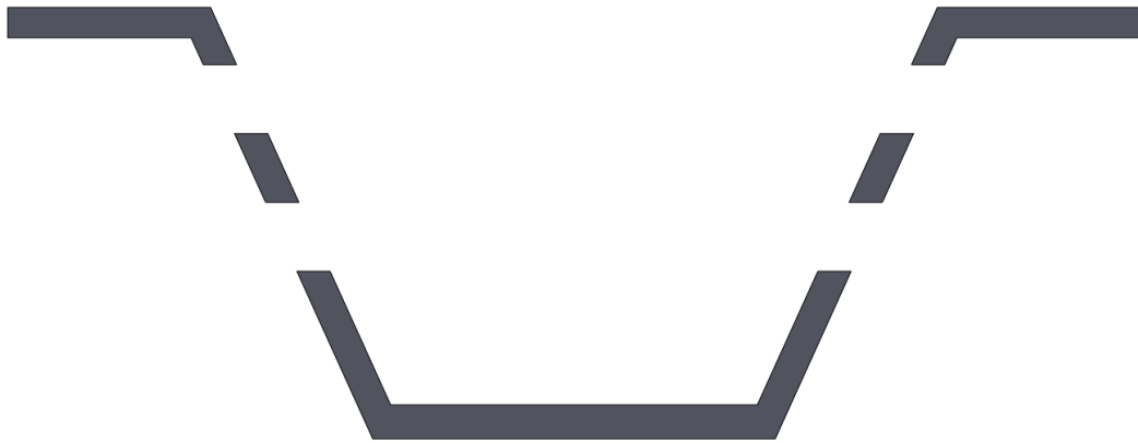
Figure 62: Cross-sectional model of the corrugated CFRTP panel
