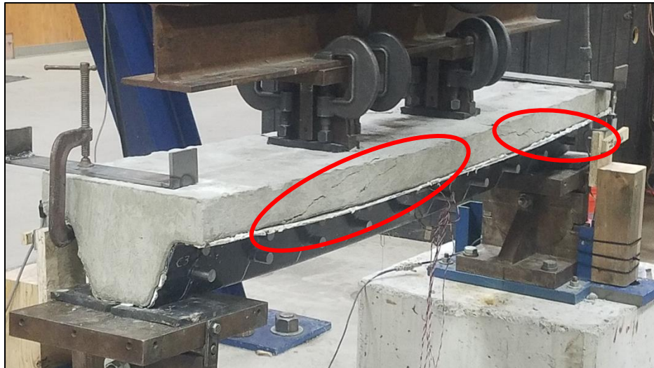
Figure 65: Shear cracks forming in the hybrid beam
