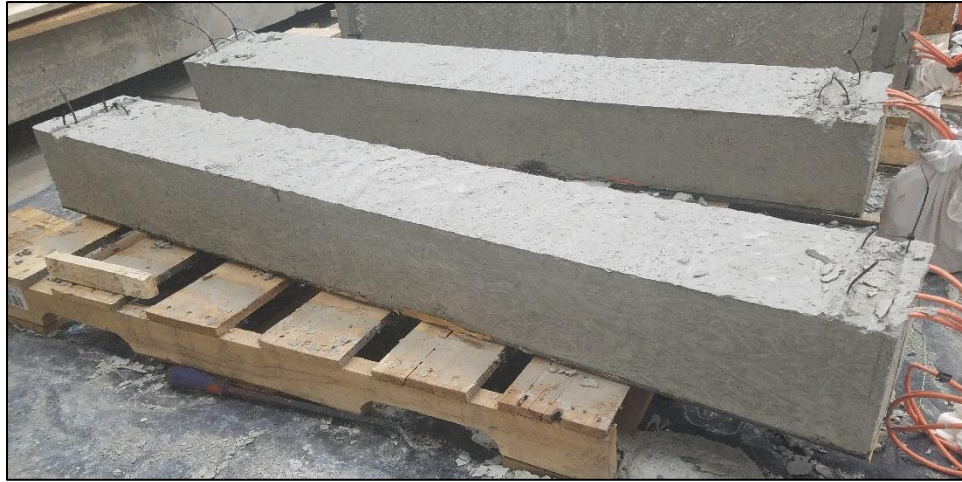
Figure 97: Composite stiffened CFRTP-concrete beam specimen, 3 days after pour
