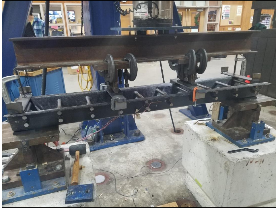
Figure 58: Construction loading test setup
