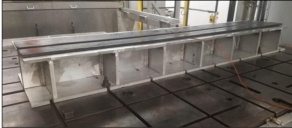
Figure A-11: Stiffeners in the mold for bonding in the hydraulic press
