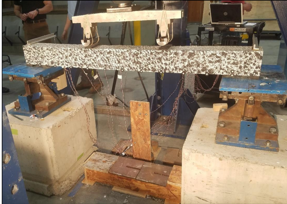
Figure 27: Hybrid flat CFRTP-concrete beam test setup
