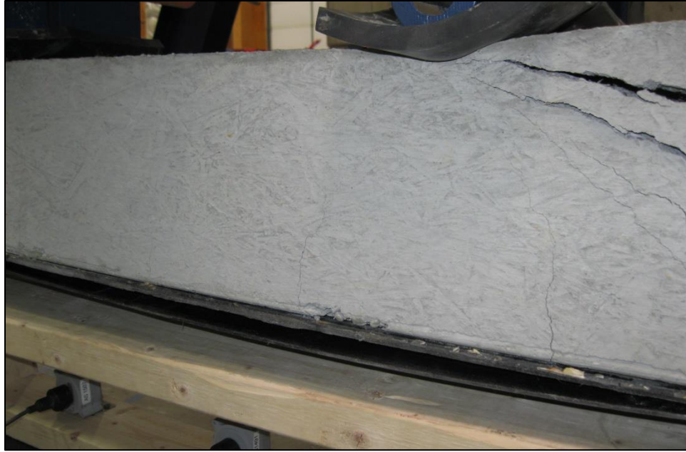
Figure 108: Broken bond between the angles and backer plate
