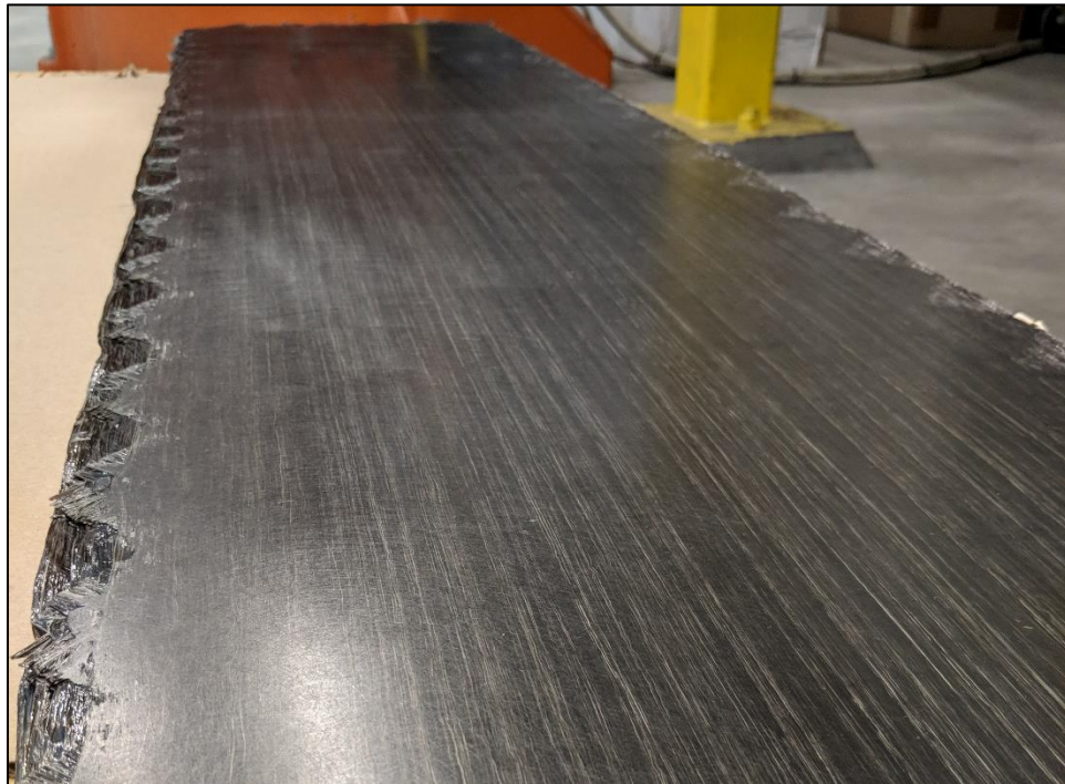
Figure 85: Consolidated panel for the angle stiffened panel
