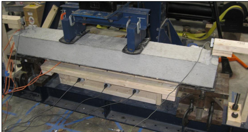
Figure 105: Ultimate Loading Test Setup
