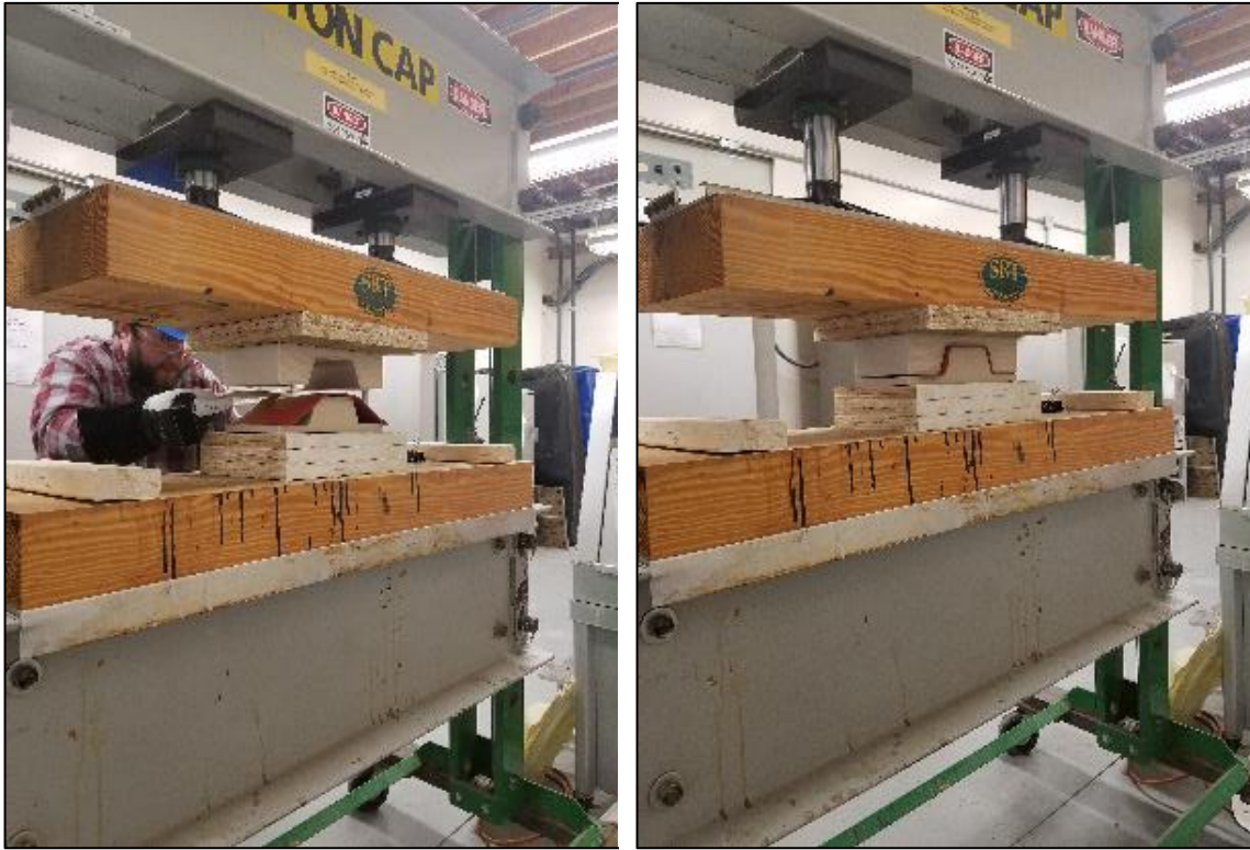
Figure B-13: Heated PETg put into the press (left) and the press closed (right)
