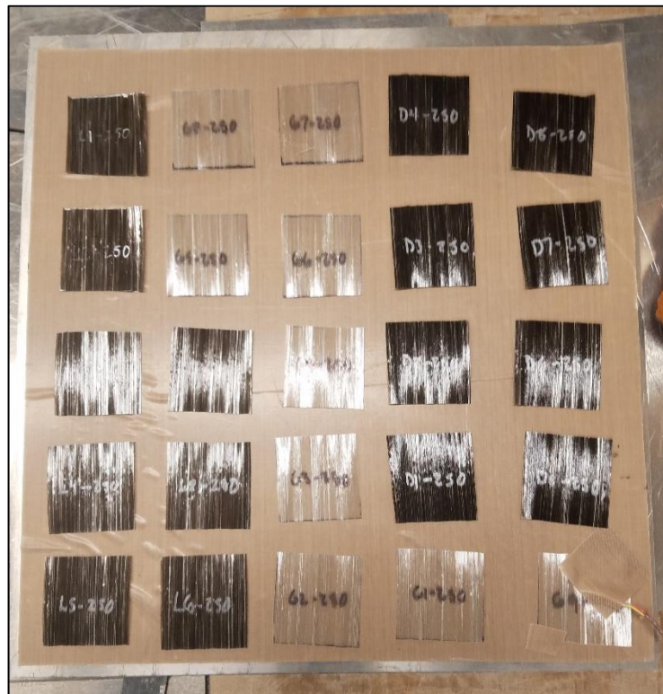
Figure B-4: Arrangement of shrinkage test specimens
