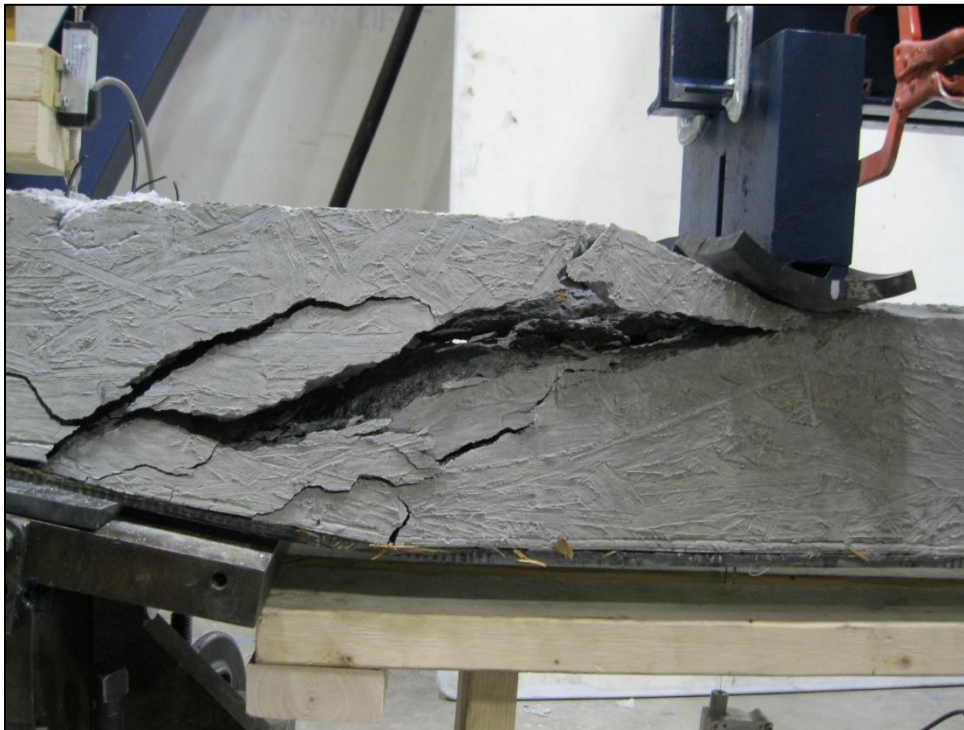
Figure 106: Shear cracks forming in the hybrid beam
