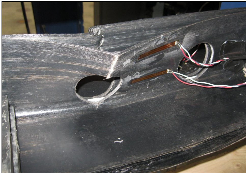
Figure 103: Initial Buckling of Specimen 2
