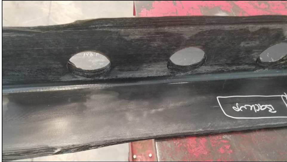
Figure 93: Observed issues with the first stiffened panel forming method
