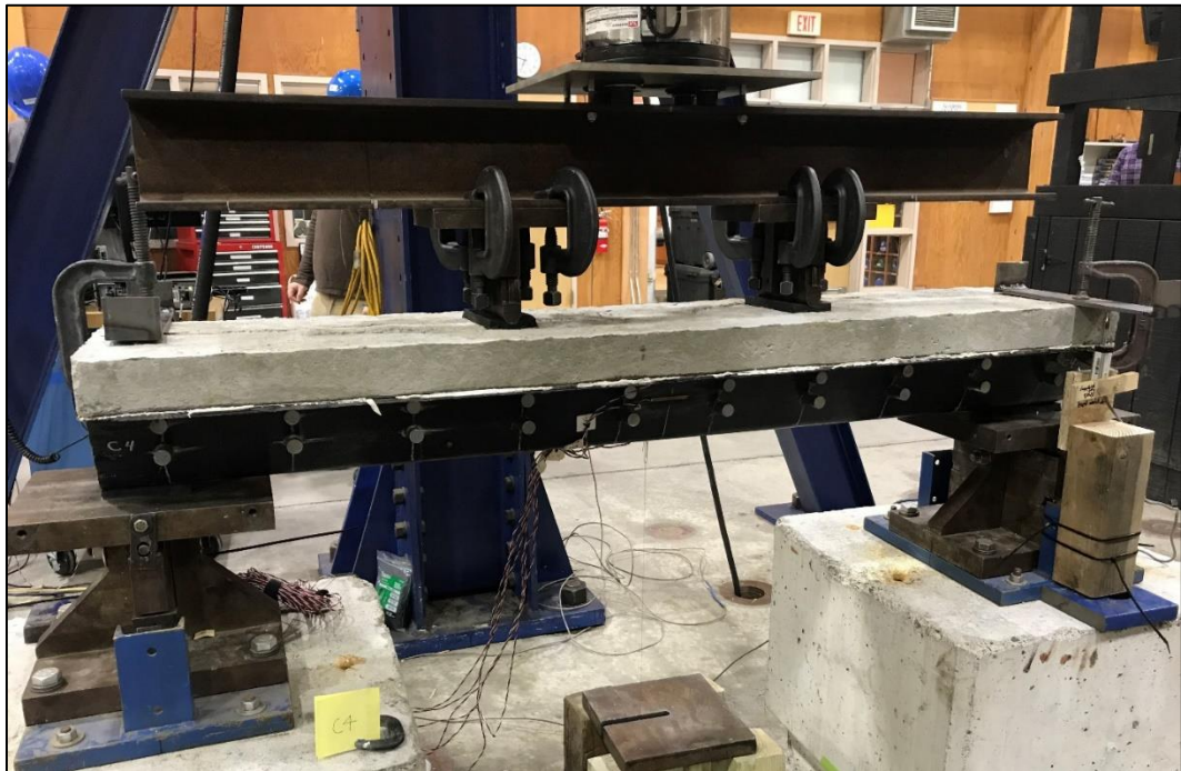
Figure 64: Ultimate loading test setup
