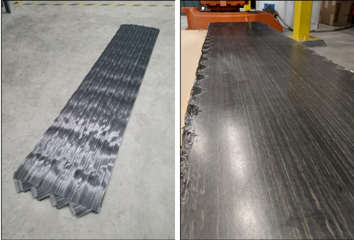
Figure A-9: Tailored blank, before (left) and after (right) consolidation
