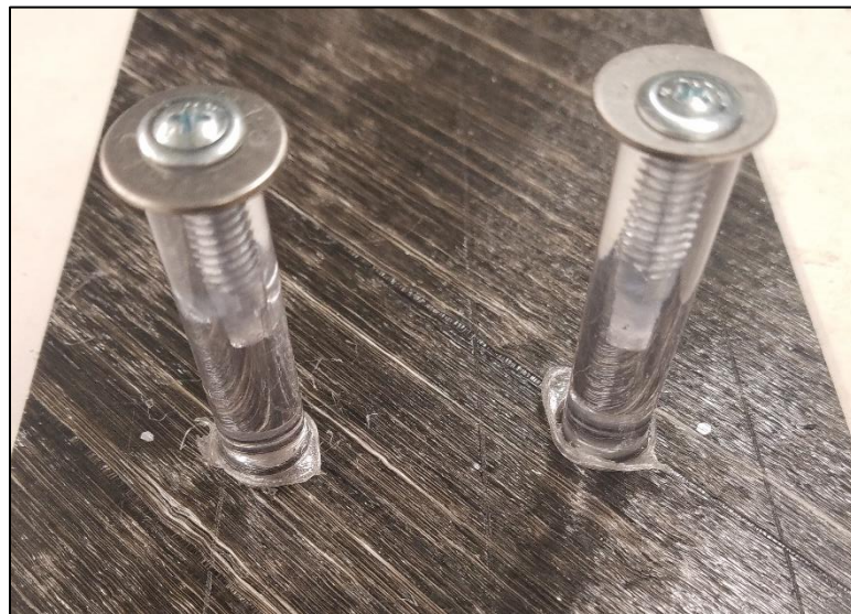
Figure 24: Flat CFRTP panel with shear studs at 152 mm spacing
