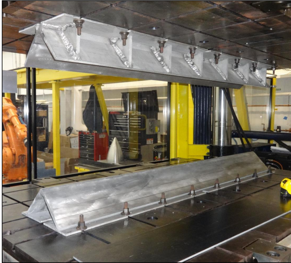
Figure 86: Angle mold in the hydraulic press
