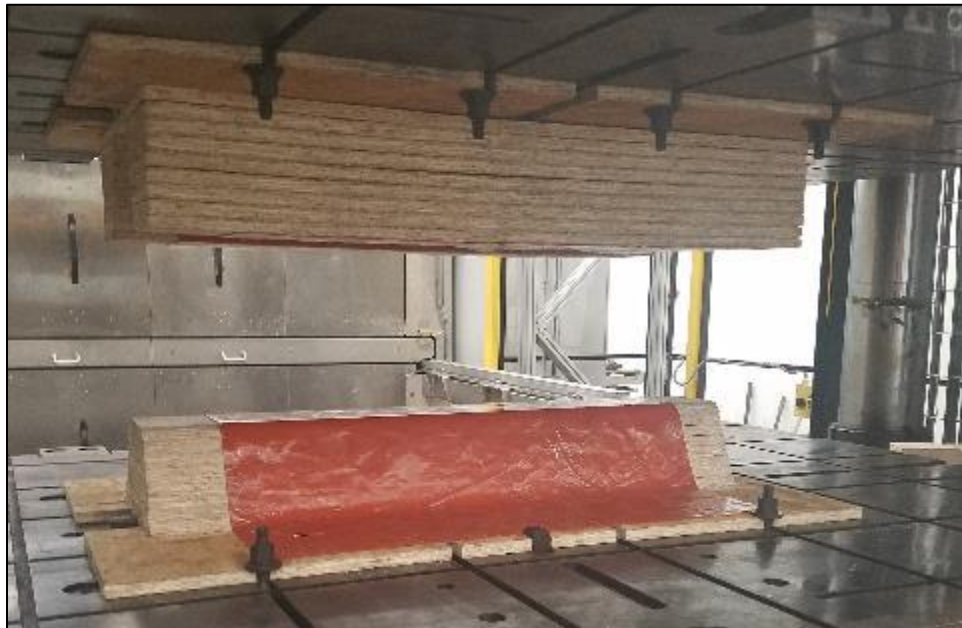
Figure B-24: OSB Corrugated mold mounted in the hydraulic press
