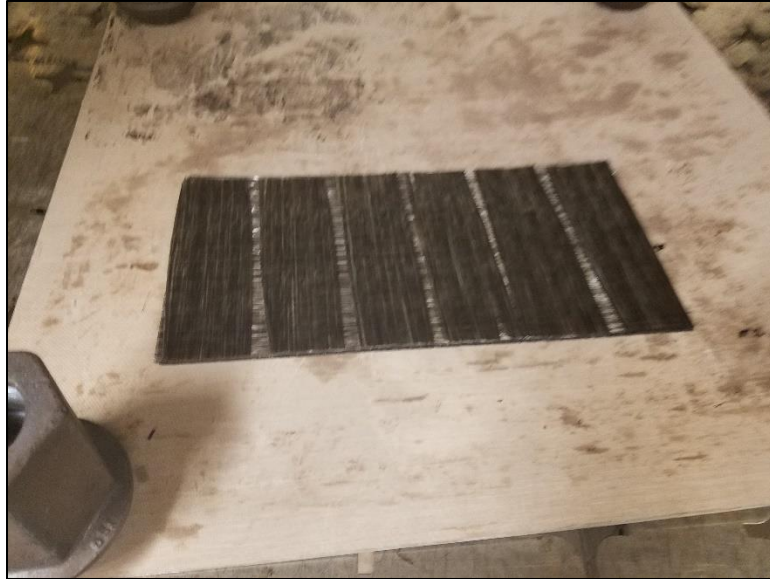
Figure B-2: Gaps observed after heating of tailored blank
