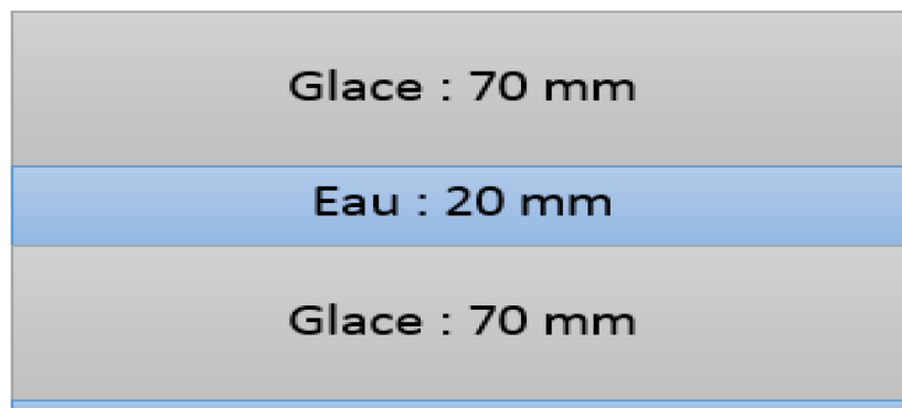
Figure 4.3 Bloc multicouche glace-eau-glace
