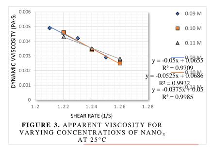
does not include the average marker indicating that this concentration of sodium nitrate experienced turbulence. The data points for the 0.09 M concentration do not lie within the normal range for human blood viscosity. The trials employing 0.10 M NaNO3 and 0.11 M NaNO3 had similar ranges and averages with little
