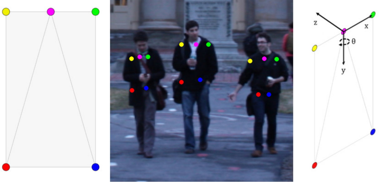
Figure 4.2: To accurately localize 2D ground points for detected people, a planar torso model in 3D (left) is first fit to detected 2D neck, shoulder, and hip joints (middle-left). Right: Coordinate axes for the planar model.
