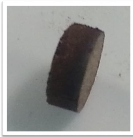
Figure 5-2: Browning and blackening of pellet one due to oxygen during sintering
