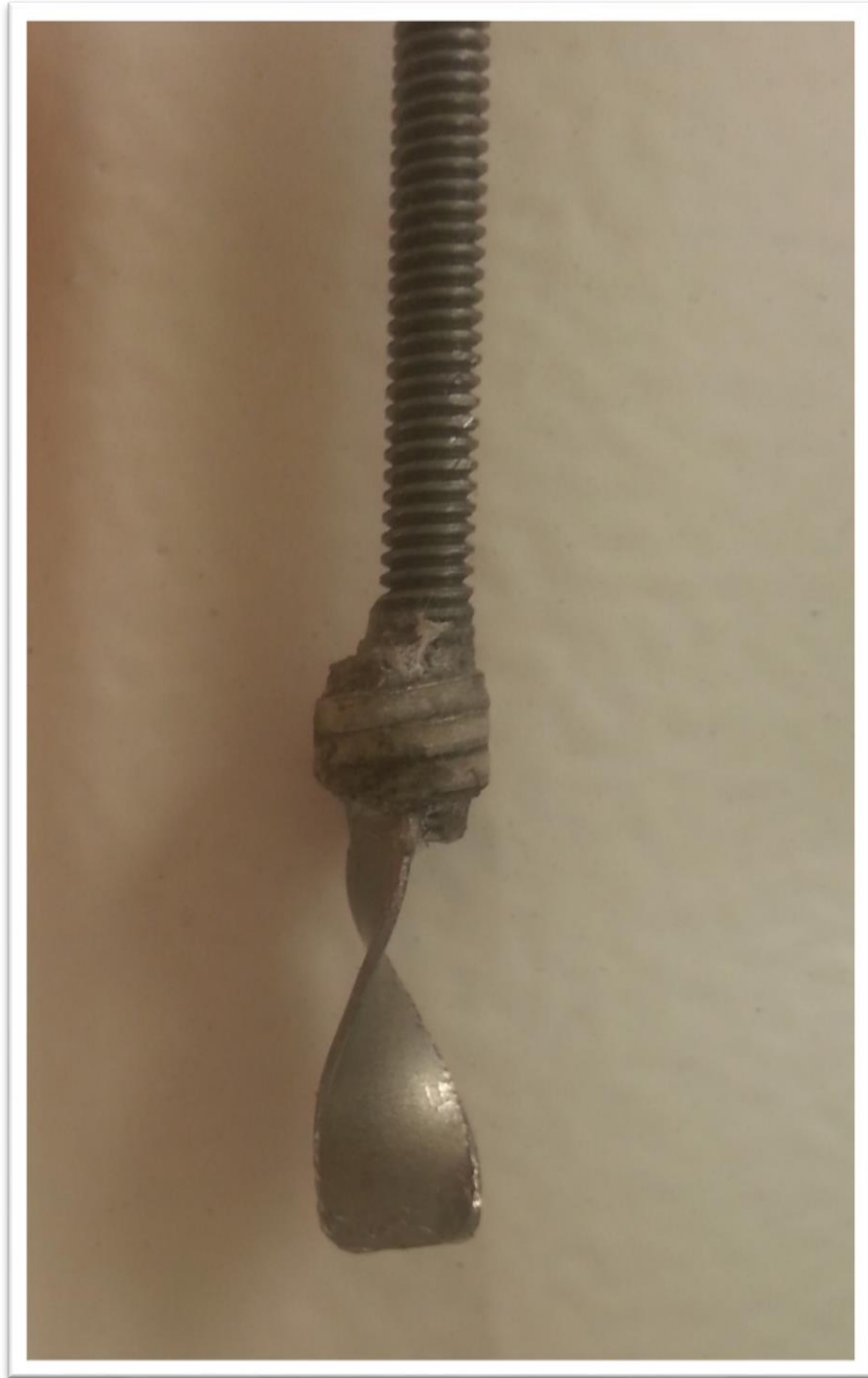
Figure 3-9: In-die stirring rod
