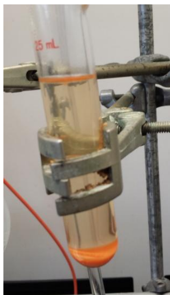
Figure 14: The nanoparticles of ZrP-Rh settle at the bottom of the Schlenk flask after combining ZrP nanoplatelets with \text{ClRh}(\text{PPh}_3)_3 .
