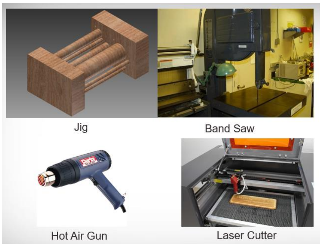
Figure 10. Tools and Machines for Fabricating Runoff Prototypes
