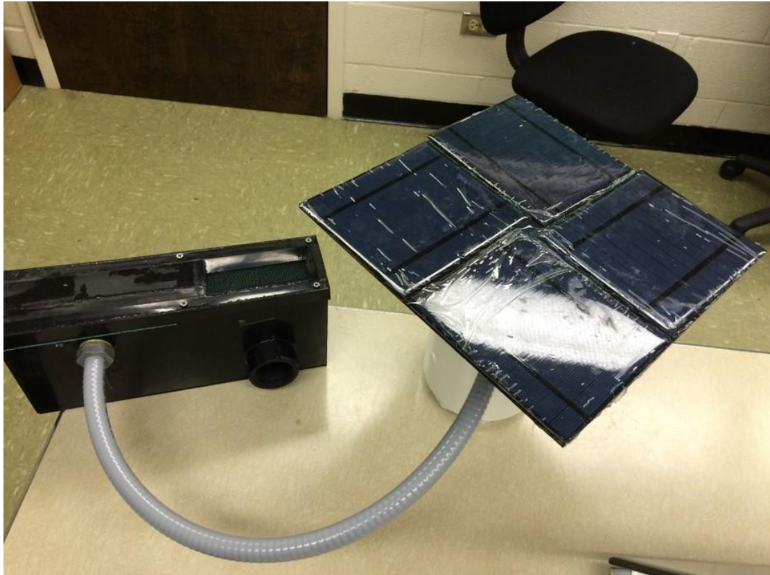
Figure 17. A Cubic Float Prototype Equipped with an Energy Supply Module
