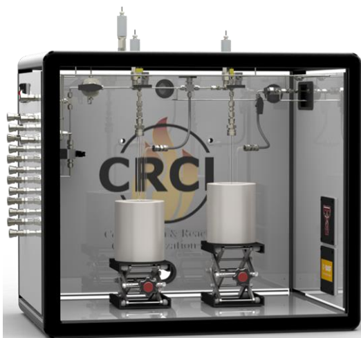
Figure 5: Microreactor Solidworks model. Gas input is on the left. Reactor 1 (sample location) and reactor 2 (oxidation catalyst location) are shown by the glass tubes just above the white, cylindrical, temperature controlled furnaces. Gas output is shown on the right.
