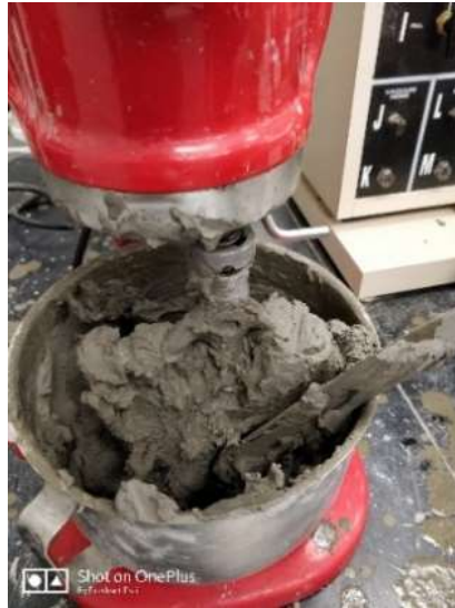
Figure 2 Soil and Grout Mixing in a Mixer
