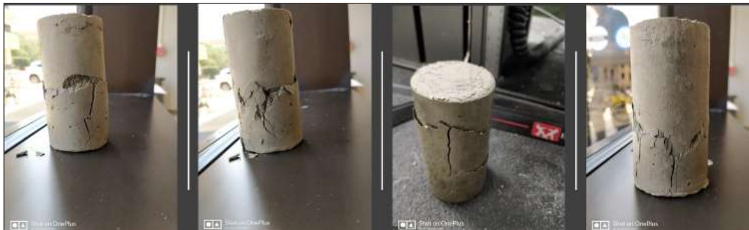
Figure 4 Specimen Failed in Unconfined and Confined Compression Test
