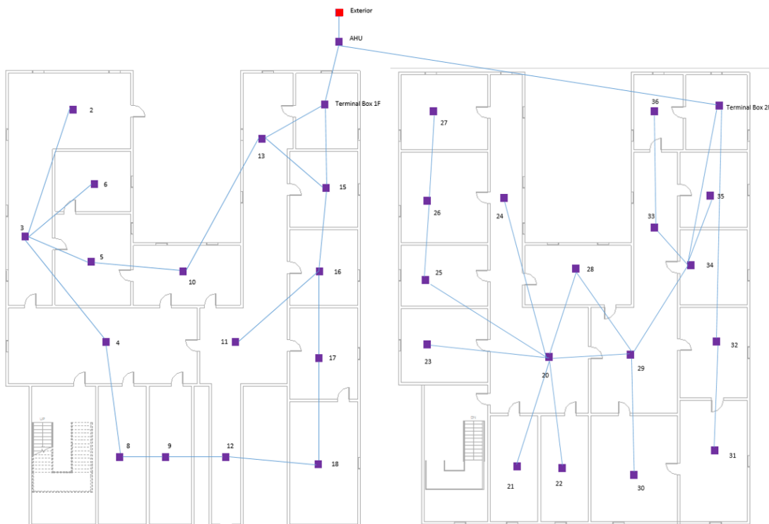
Figure 20. The connectivity study of the HVAC system in the hospital
