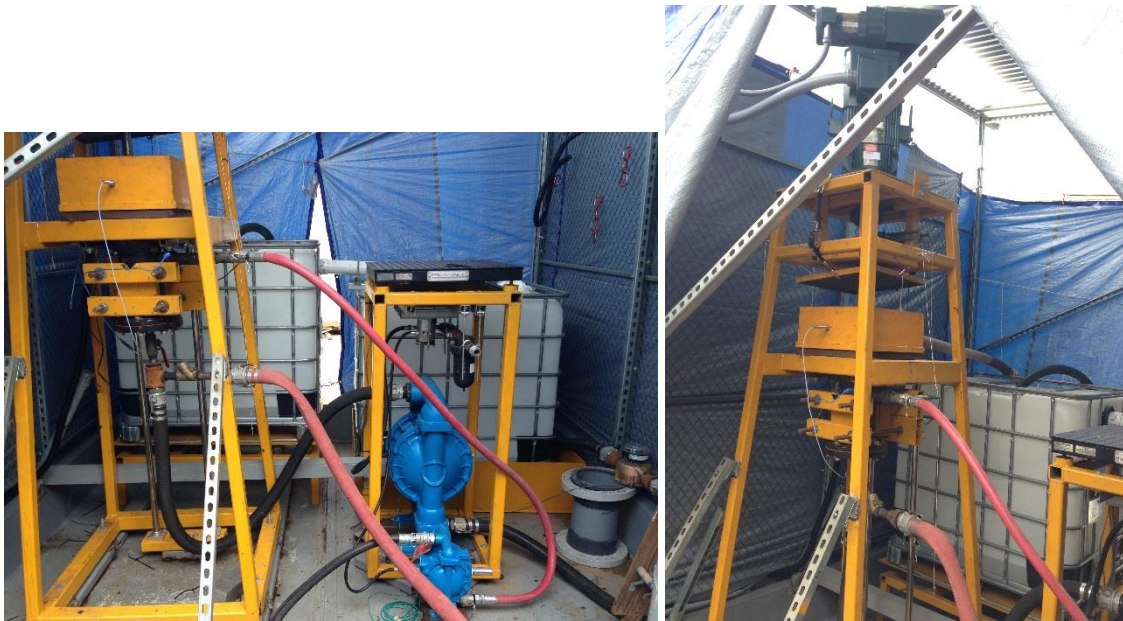
Figure 2-28 Vertical bearing/seal test rig
