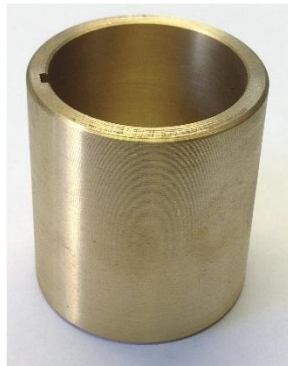
Figure 3-1 Brass journal used in the experiments
