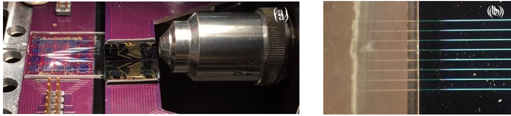
Fig. 65 On-chip optical coupling portion of the setup. (a) Shows the 1x8 PLC fiber array coupled to the LiNbO 3 and Si 3 N 4 chips and (b) shows a zoomed in vertical view of the edge coupling of the LiNbO 3 and Si 3 N 4 chips [21].
