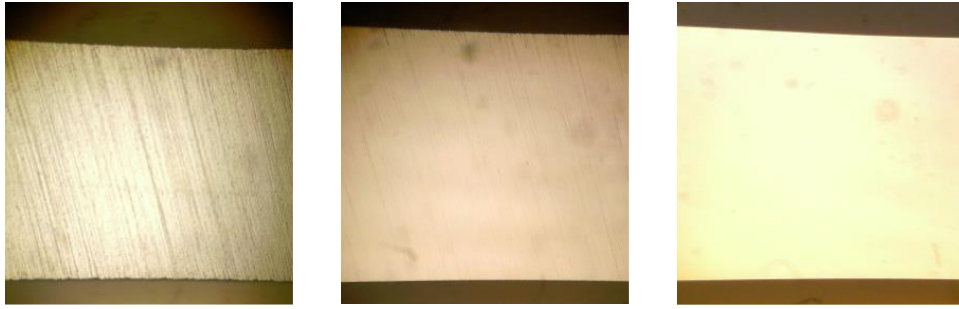
Fig. 33 Edges of sample after polishing with the a) 15 \mu m, b) 3 \mu m, and c) 0.5 \mu m pads, respectively.
