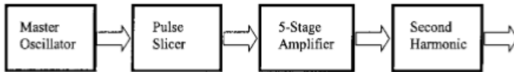
Figure 2.8 Basic outline of a pulse-burst laser system. Reprinted from [37]
