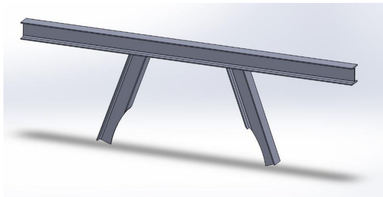
Figure 24. Tube support for mixing system piping manifold.
