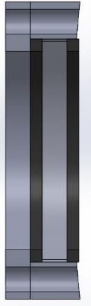
Figure 40. Profile sectioned view of oval window, showing curve of tube-side attachment.
