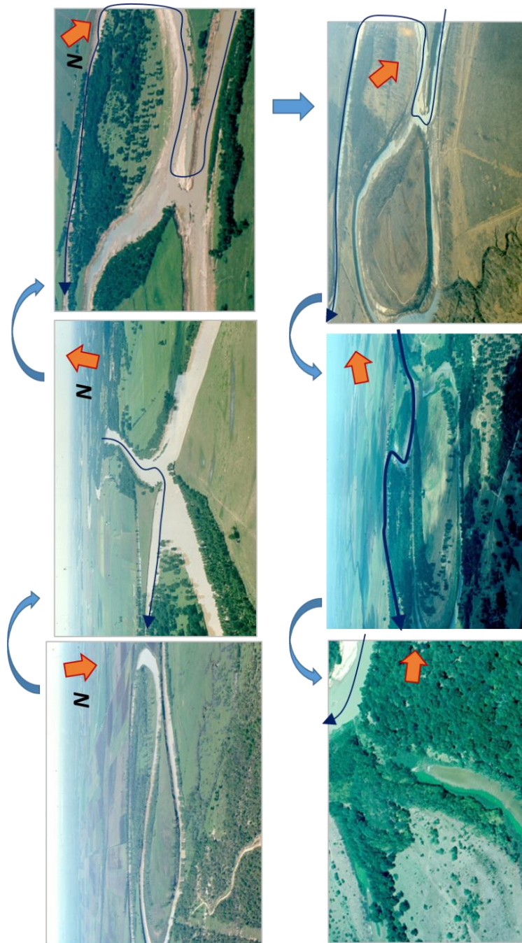
Figure 4.6 Oblique aerial photographs of cutoff of Big Bend Oxbow near College Station, Texas (Aerial photographs provided by C. Matthewson, Texas A&M University). The cutoff occurred approximately in 1974 and by the late 1970s the majority of the arms of the oxbow had infilled with sediments. The main channel is approximately 100 meters wide.
