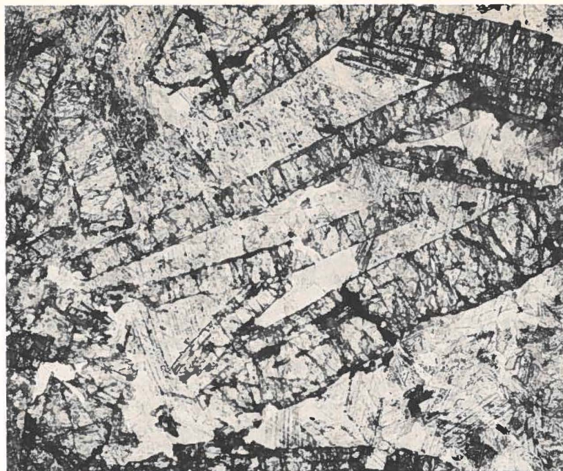
FIGURE 4. Photomicrograph of tabular bastnaesite crystals in calcite matrix. (25x, plane polarized light)
