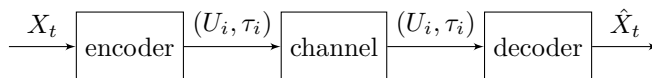
Figure 1: System Model. Sampling time \tau_i and codeword U_i are chosen by the encoder’s sampling and compressing policies, respectively.
